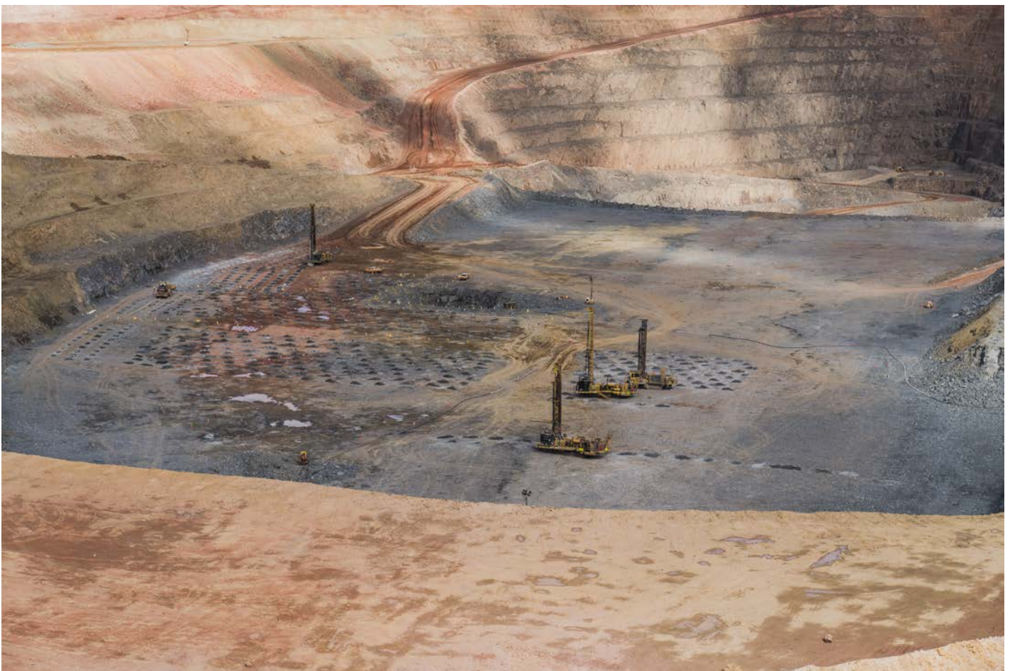
Blast hole drilling at Gruyere JV gold mine open pit
