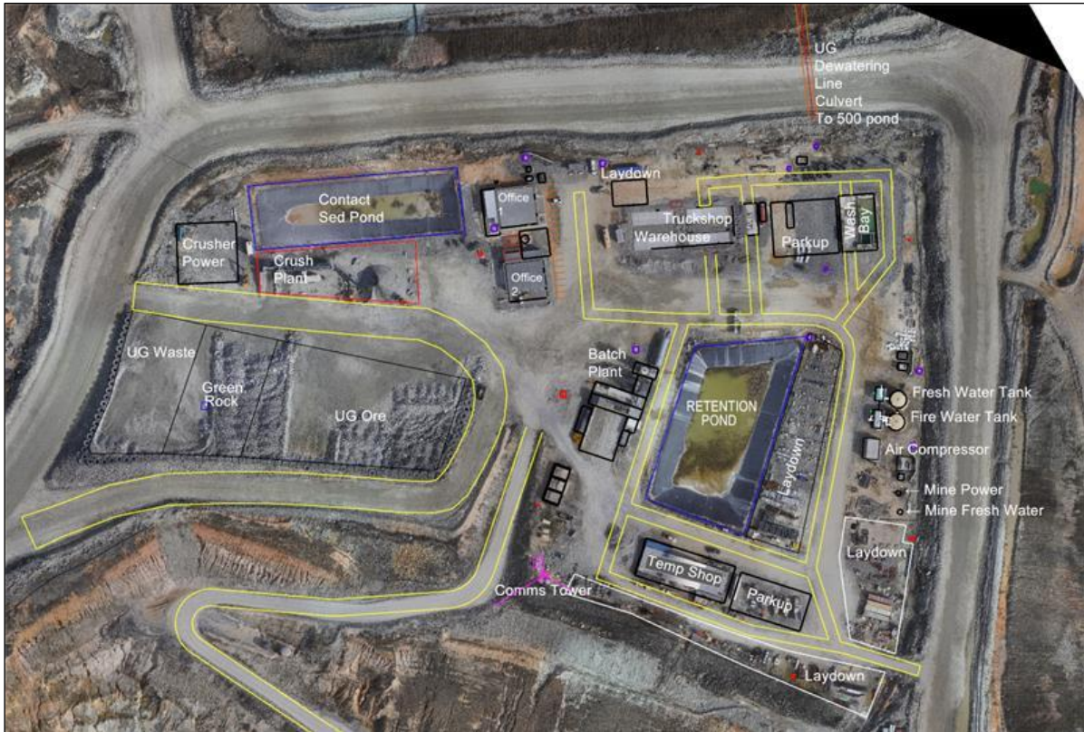
Figure 18-8: Underground Surface Infrastructure Detail
