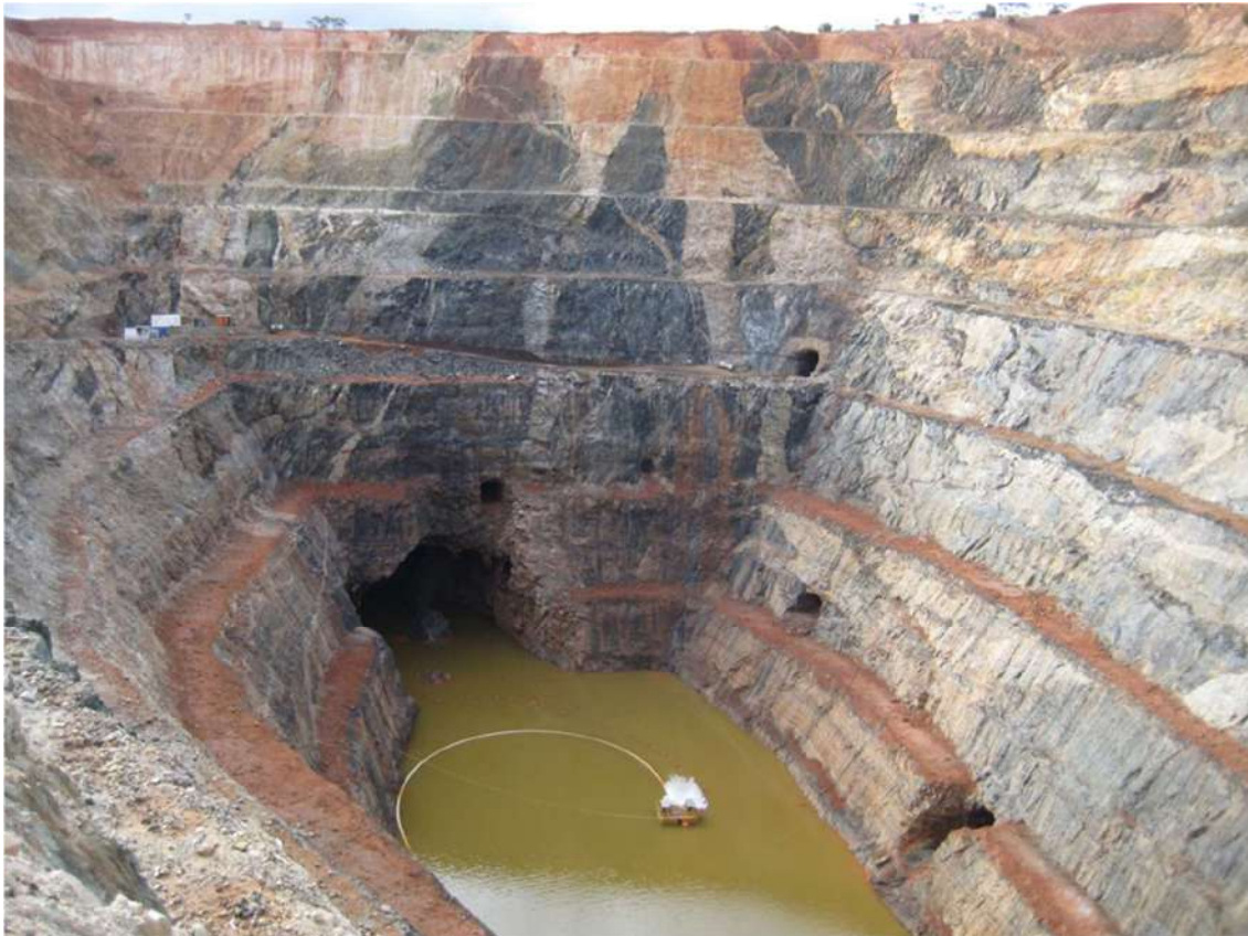
Figure 16-10 North wall of the Chalice pit showing the three main lithological zones, granite, ultramafic and amphibolite, along with various intrusive
