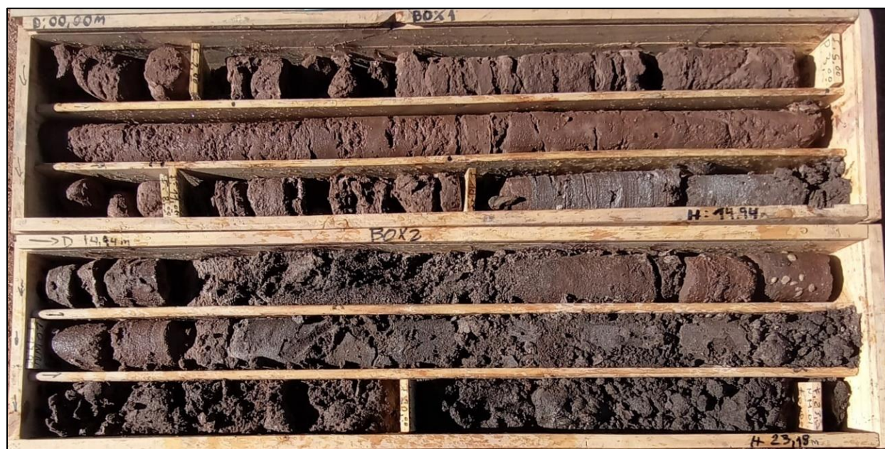
Figure 7-11: Interlayered Fine and Coarse Sediments (IFCS) in Natalia Maria, with Ulexite Crystal at Approximately 15.5 mbgs (DDH-AS23-01, 0.00-23.18 mbgs)
