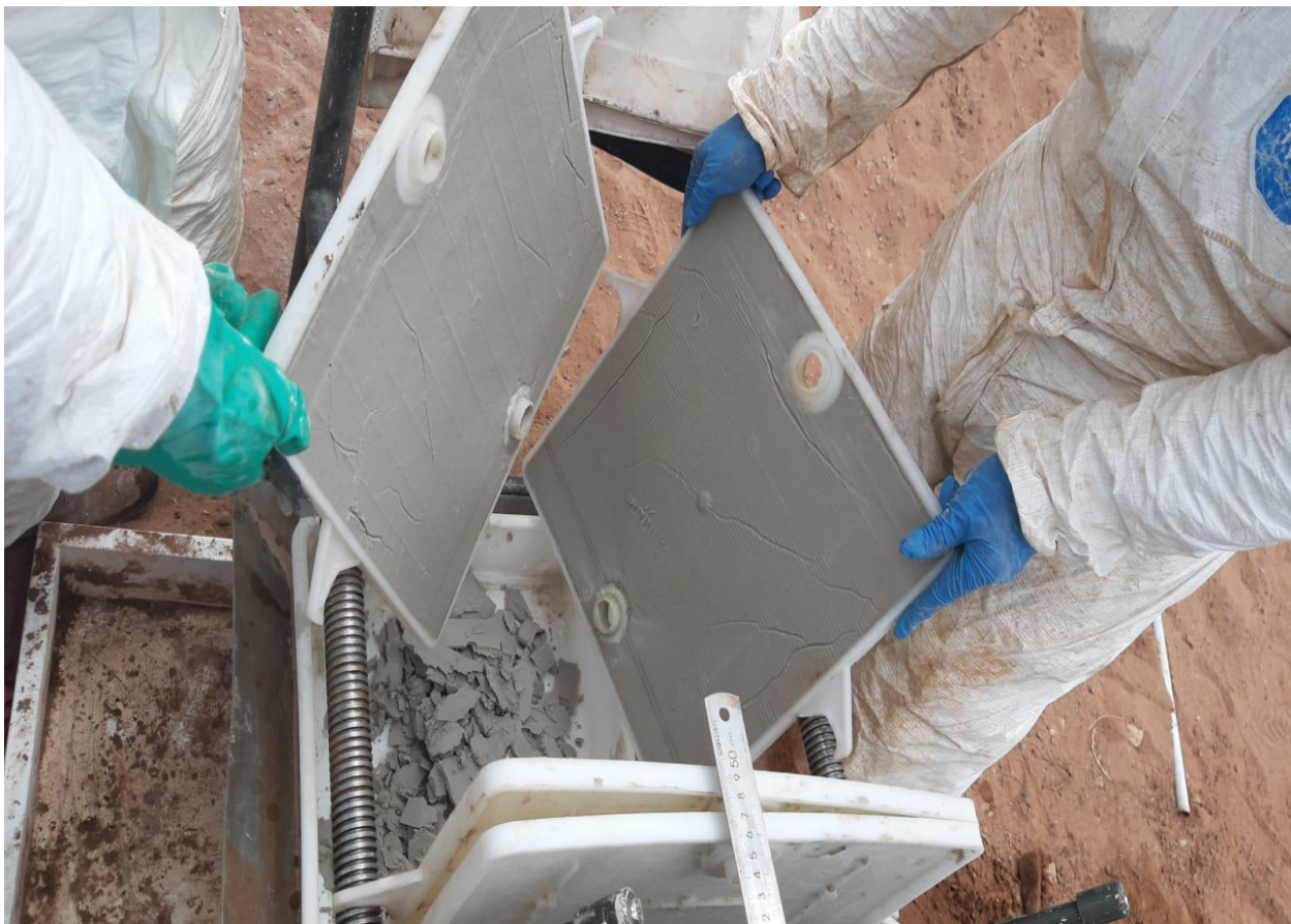
Figure 13-7: Mechanical Separation after Liming
