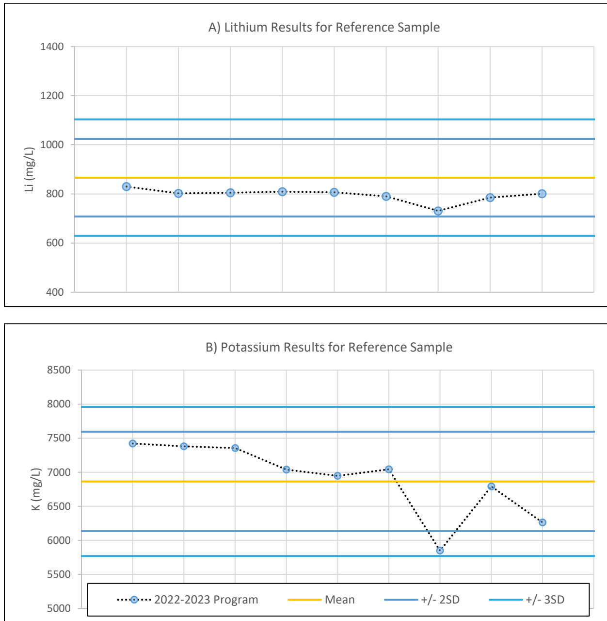
Figure 11-4: Reference Sample Results Compared with Round Robin Mean and Standard Deviation for A) Lithium and B) Potassium
