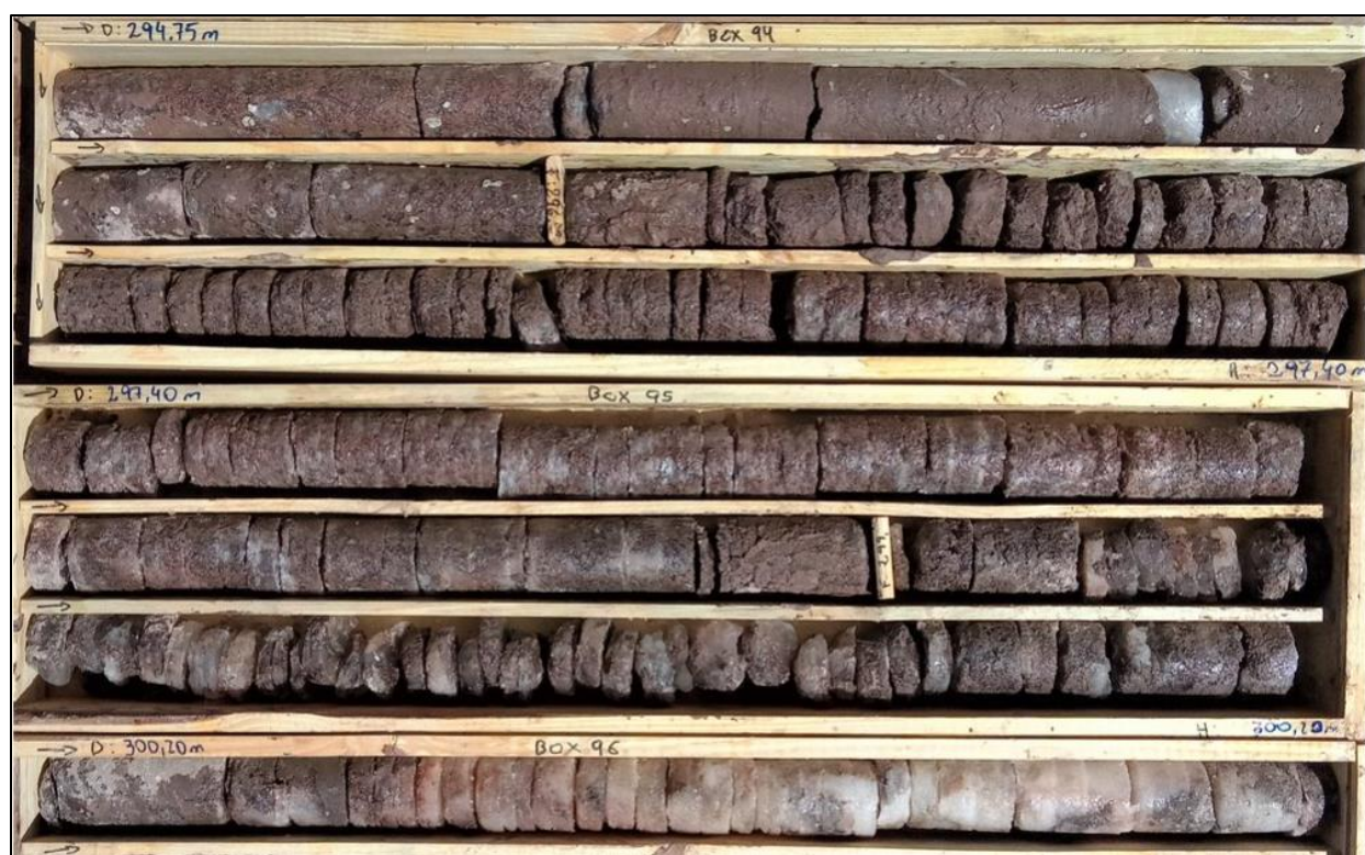
Figure 7-9: Compact Halite (CH) with an Approximately 1 m Thick Medium Grained Sand Interlayer at Natalia Maria (DDH-AS23-01, 294.75-301.0 mbgs)
