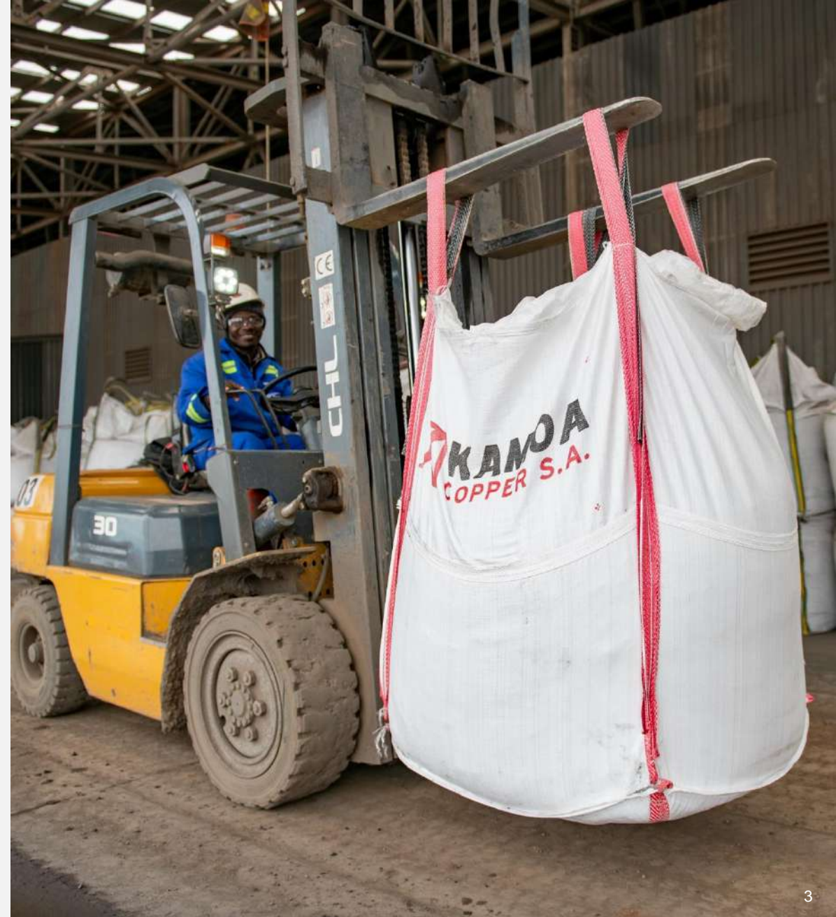
2 tonne bags of copper concentrate ready for export. Kamoia-Kakula's concentrate is one of the highest grade in the world, at approximately 50% contained copper. It is currently shipped to smelters all over the world
