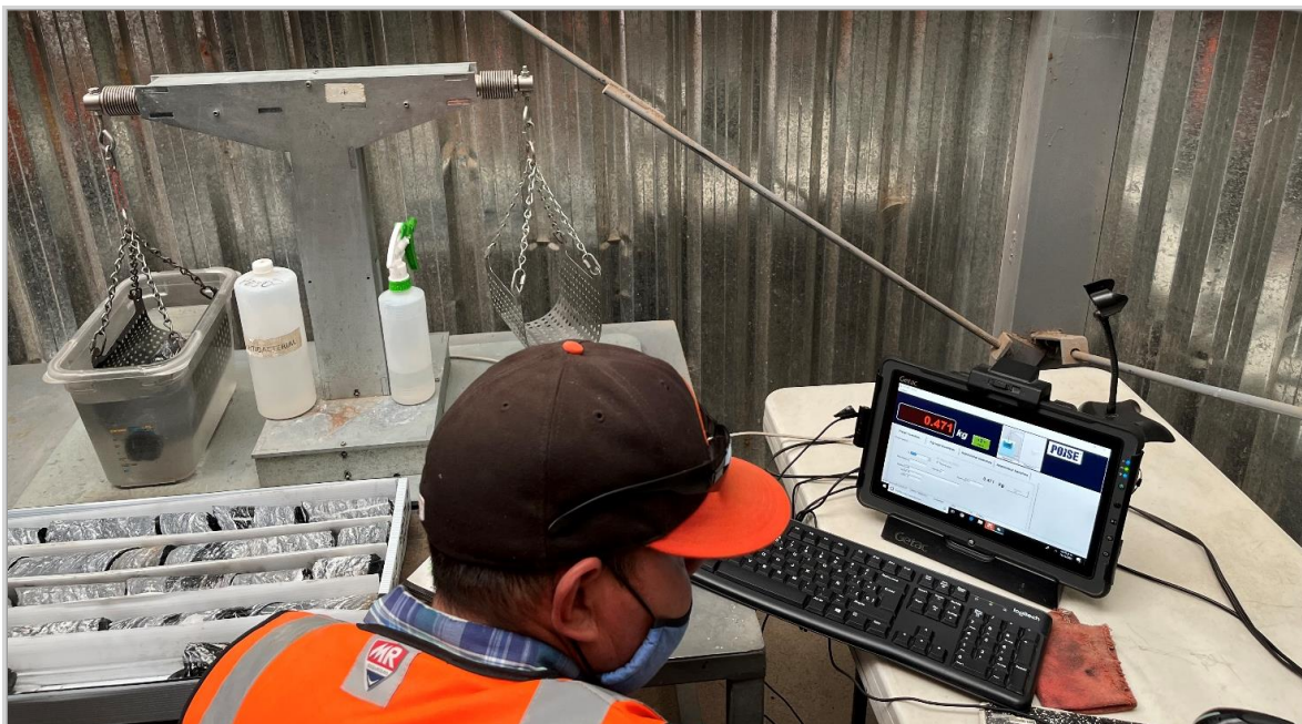
Figure 11.1 Density measurement station with electronic scale and instrument to record data
