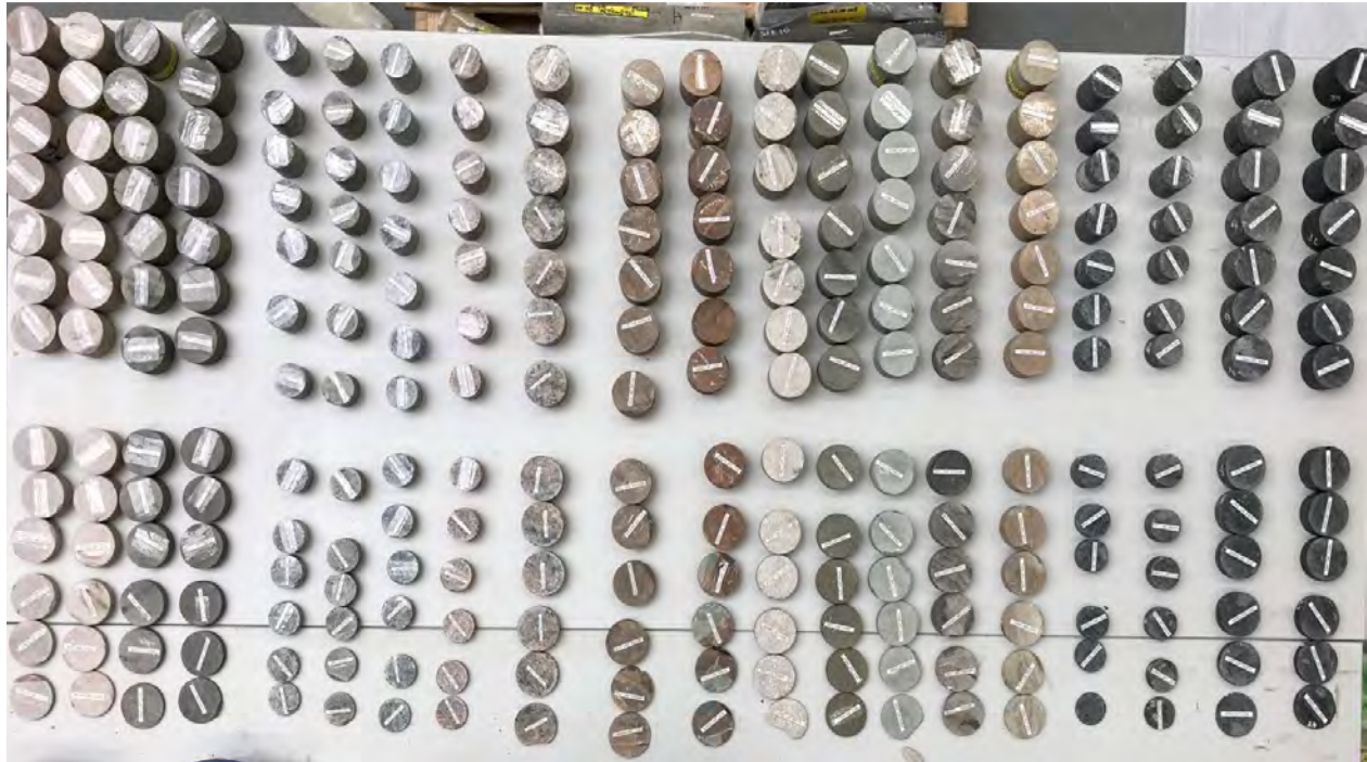
Figure 13-1: Ore and Waste Samples Prepared for XRT Testing
