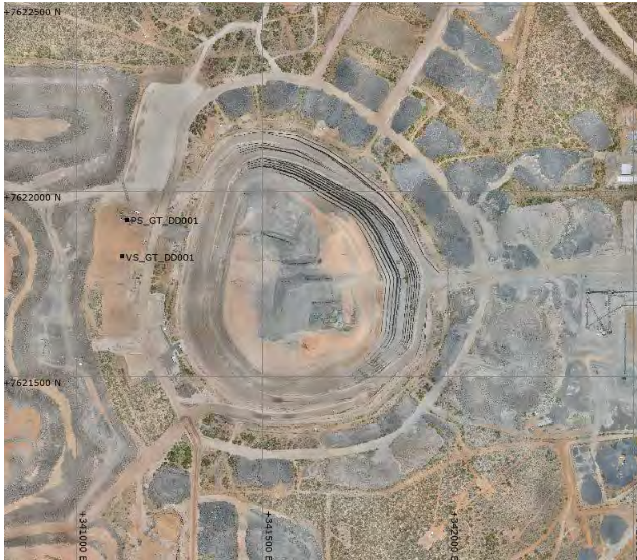
Figure 10-3: Geotechnical Drillholes of Proposed Shafts
