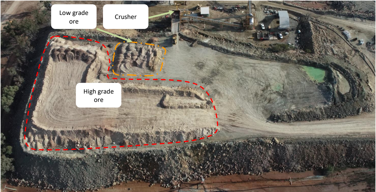
Figure 4: Stockpiled oxide ore on the ROM pad.
