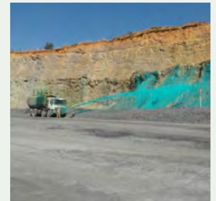
At Paracatu, spraying polymer on mine slopes.
