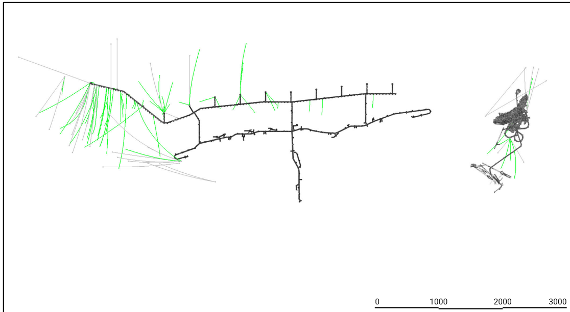
Figure 4-11: Plan view showing the layout of the exploration drift and water drift at the 1375-level and the layout for Konsuln (in black). Source: LKAB.
