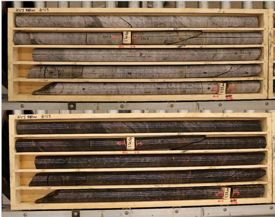
Figure 4-12: Representative Images of Drill Core Photographs in a) Dry and b) Wet Conditions.
