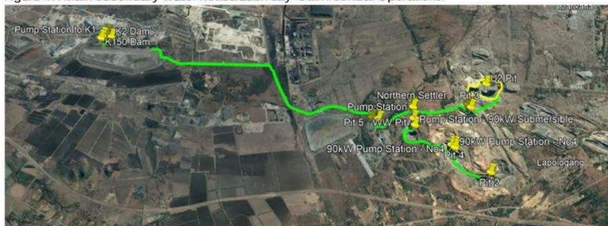
Figure 47: Main Secondary Water Reticulation Lay-Out Kroondal Operations.
