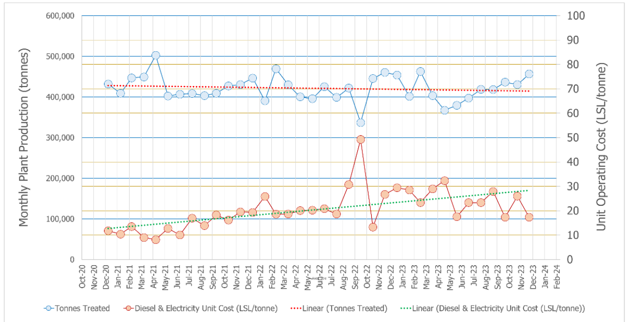
Figure 17-22: The combined monthly production tonnage and plant operating unit cost for diesel and electricity for the period January 2021 to December 2023
