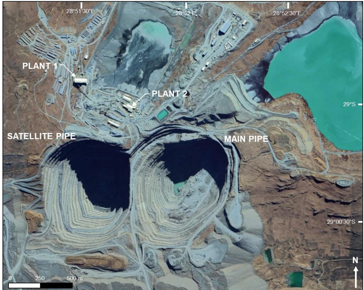
Figure 18-2: Aerial photograph of the Satellite and Main Pipe open pits and the process and recovery plants
