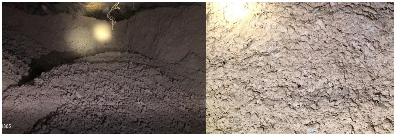
Figure 18.8: CRF Placed by Rammer Jammer in a Cut-and-fill Stope (left). A Close-up View of CRF in a Longhole Stope
