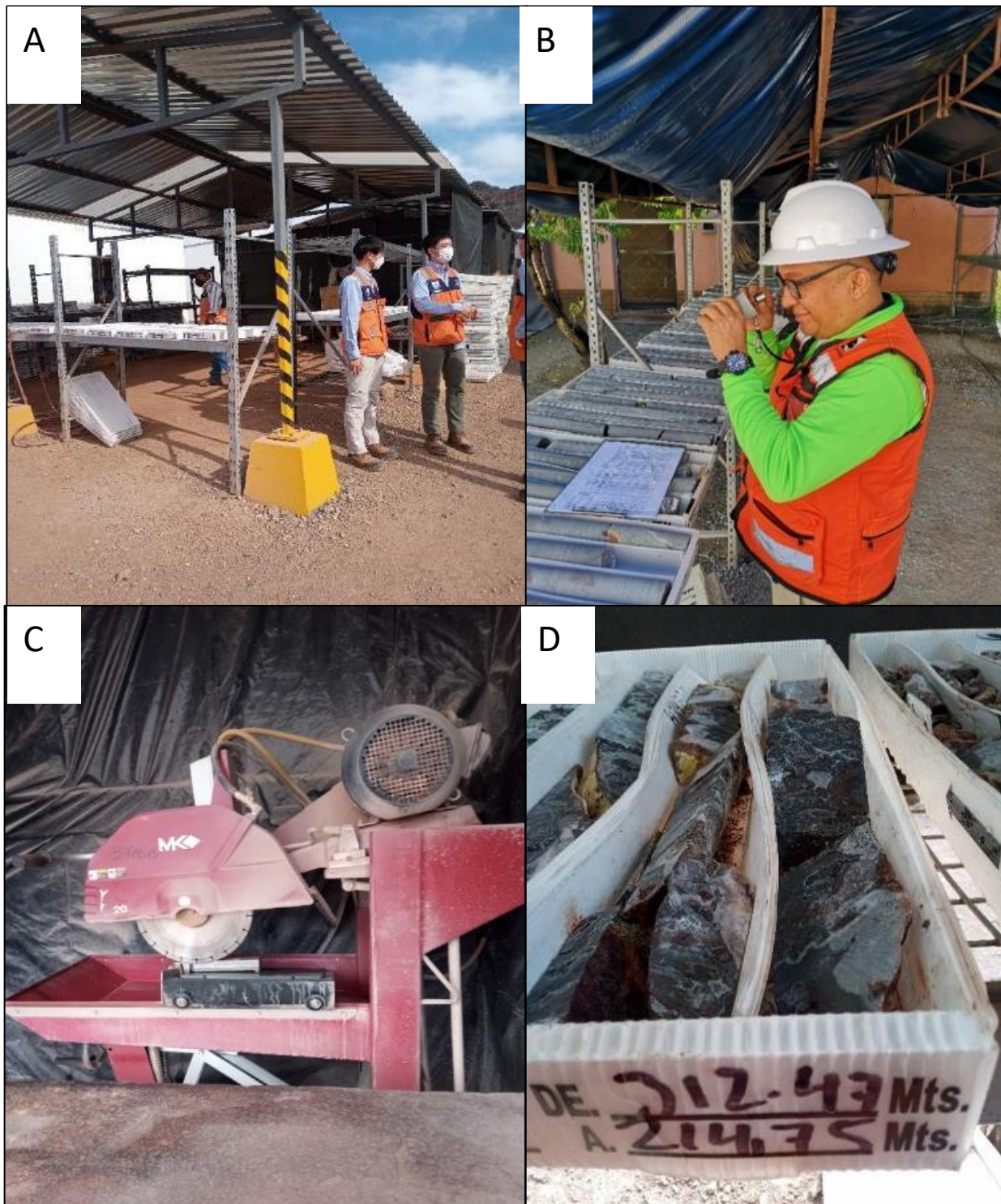
Figure 11.2: A) Geological Core-Shack; B) Geological Logging on Site; C) Electrical Diamond Saw; D) Half Core Placed in a Labelled Core Box
