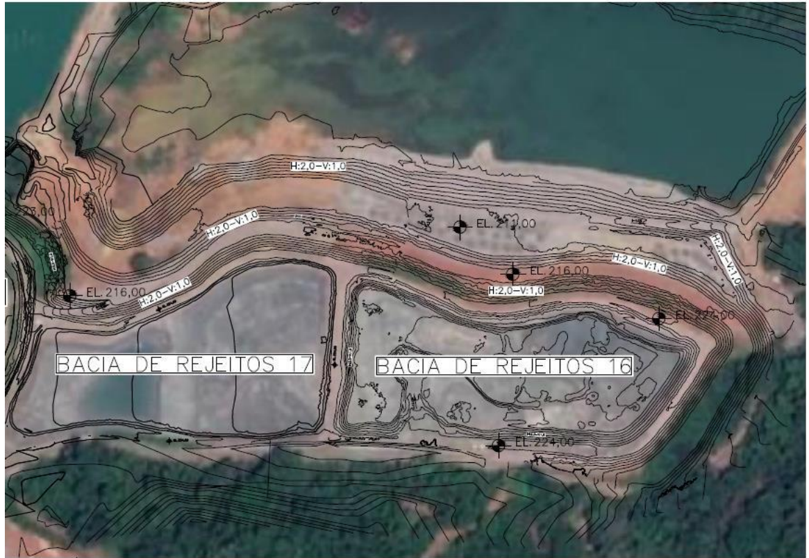
Figure 18-4: Active Tailings Dams 16-17
