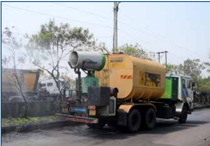
Long Range Mist Blower (Fogging Machines)
