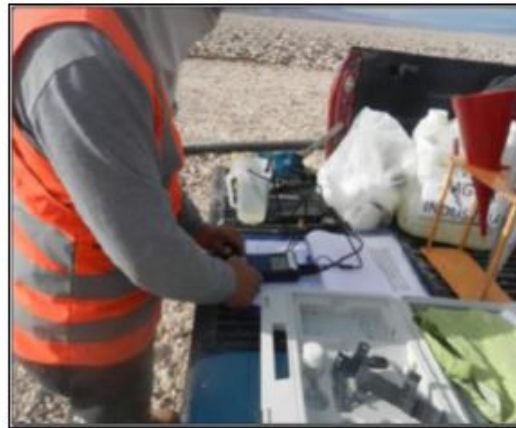
d) pH, temperature, and conductivity measurement
