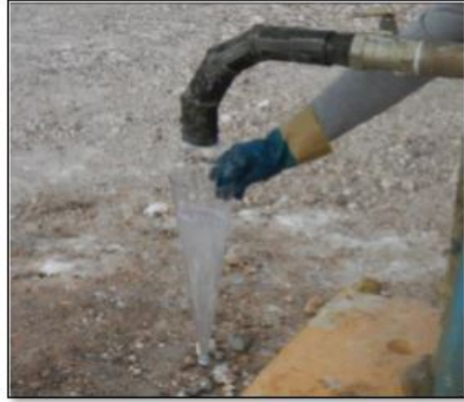
b) Clarity and fine sediment measurement
