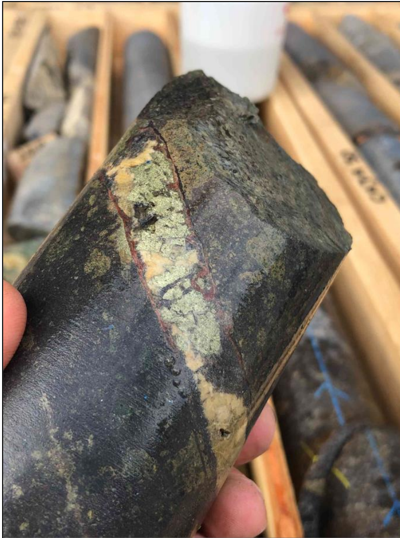
Figure 7-12: Chalcopyrite-Siderite Vein in Andesite with Pervasive Specularite Alteration (Drill Hole SJ21-07 at 152.50 m)
