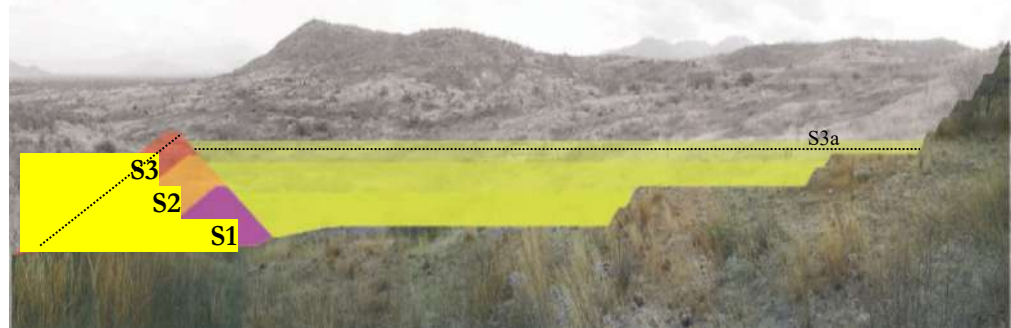
Figure 18.3 Schematic drawing showing phase 1, phase 2 and phase 3 tailings dam
