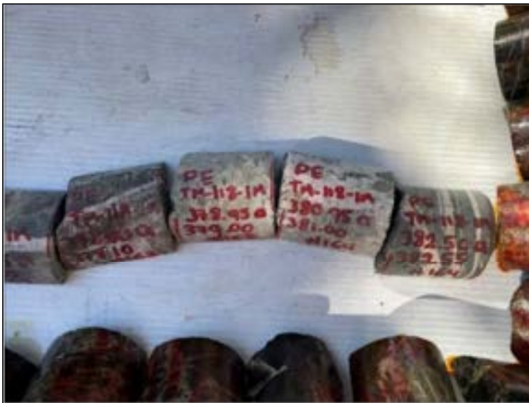
Figure 8.2: Core Samples Selected for Specific Gravity Testing
