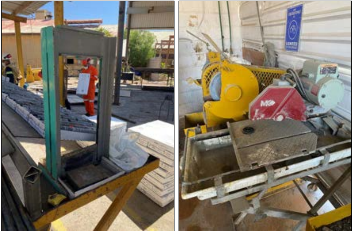
Figure 7.7: Core Splitter and Electrical Saw used at Santa Bárbara
