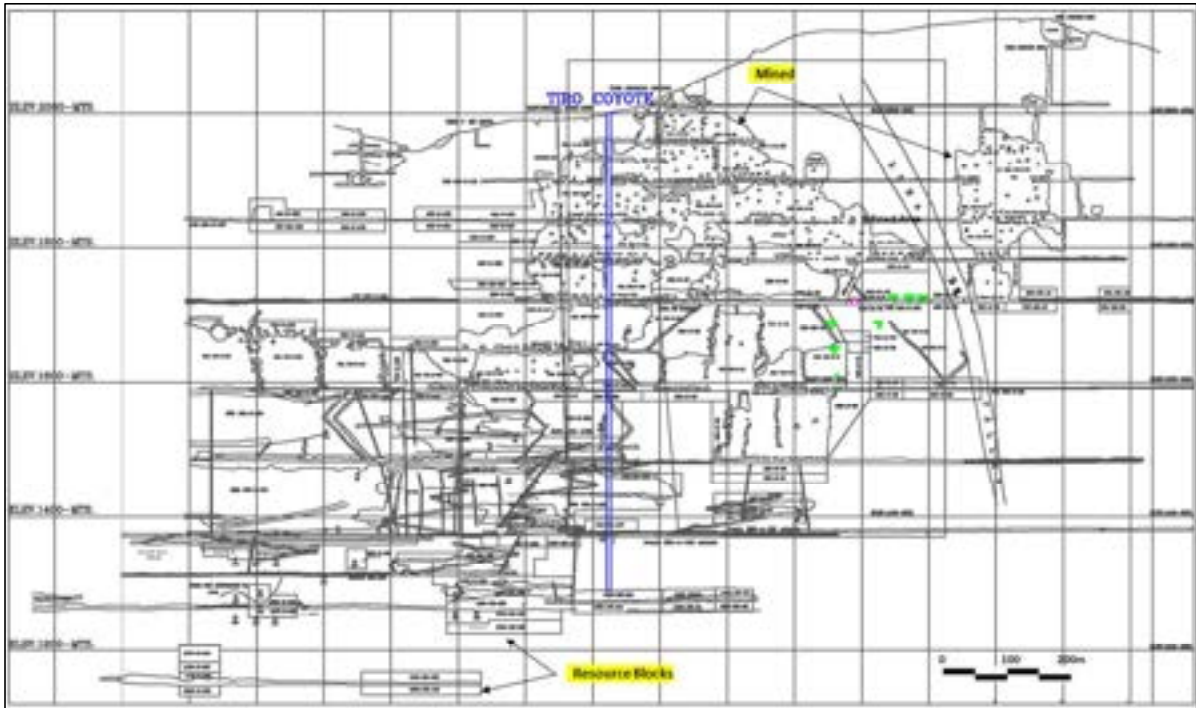
Figure 6.11: Long Section of Loteria Limpia Vein and Underground Workings
