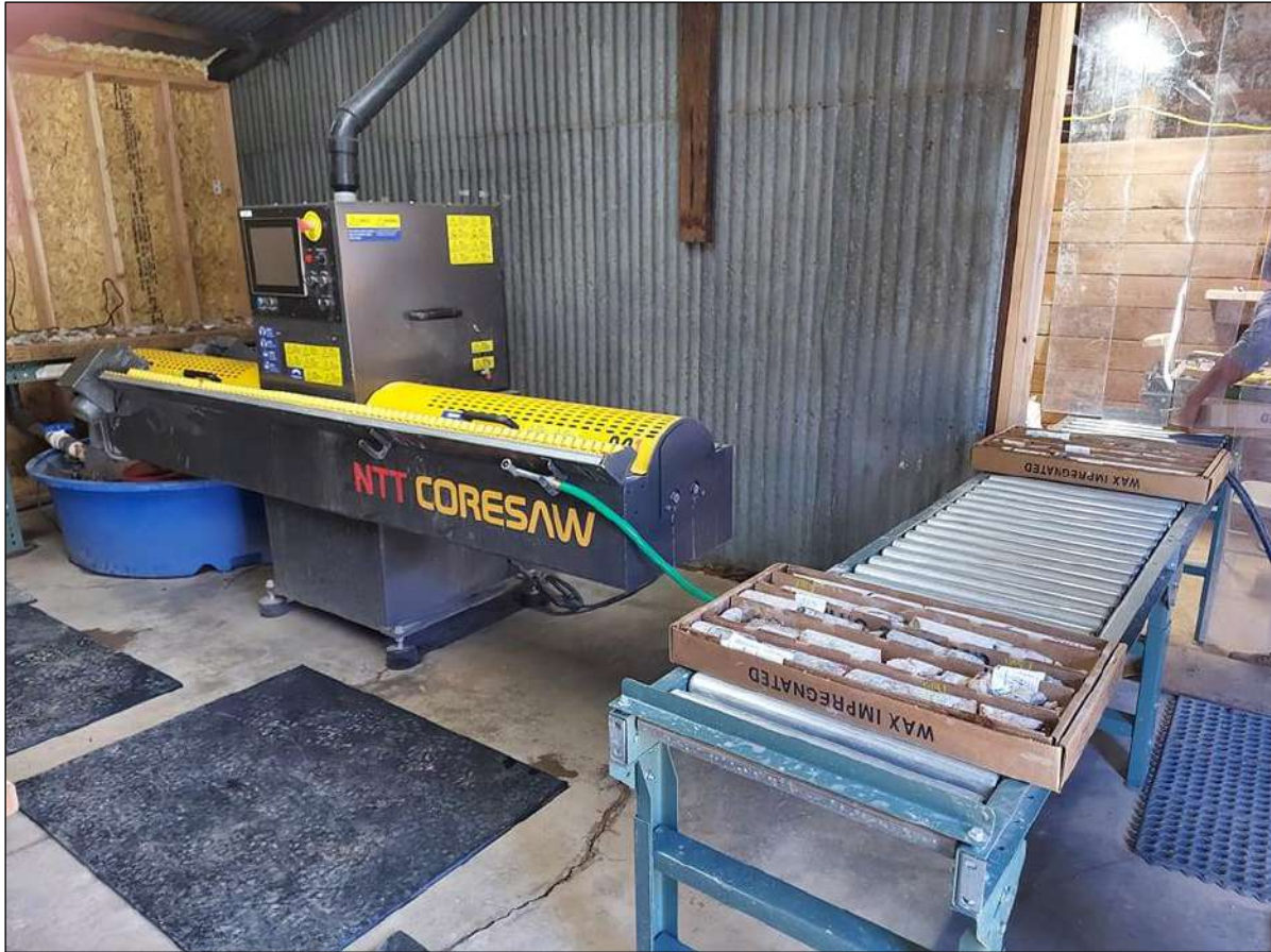
Figure 11-1: NTT Diamond Bladed Automatic Core Saw used for Cutting Diamond Drill Core for Sampling
