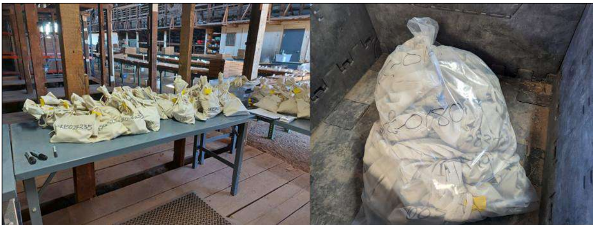
Figure 11-3: (Left) samples placed in burlap and inner plastic bags labeled with sample numbers; (Right) sample batches placed in large plastic bags and bins for shipping to lab
