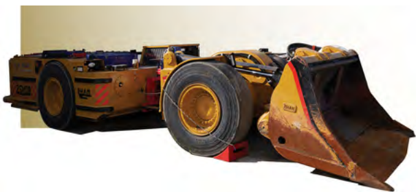
Remotely operated battery-electric LHD at the Bathopele operation at SA PGM
