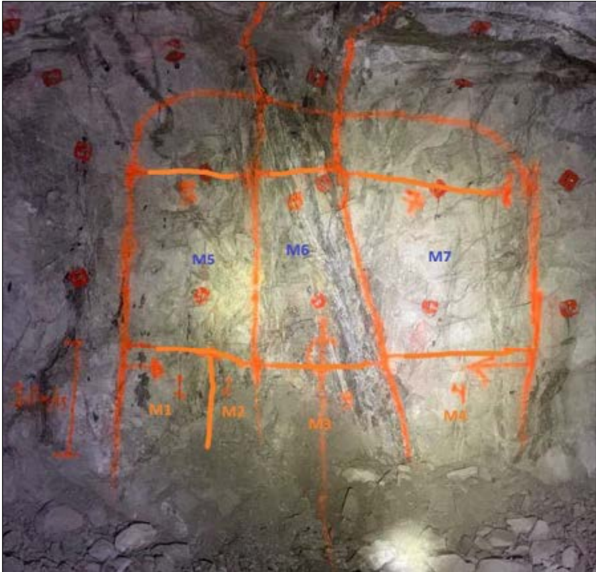
Figure 7-6: Panels Marked for Chip Rock Sampling
