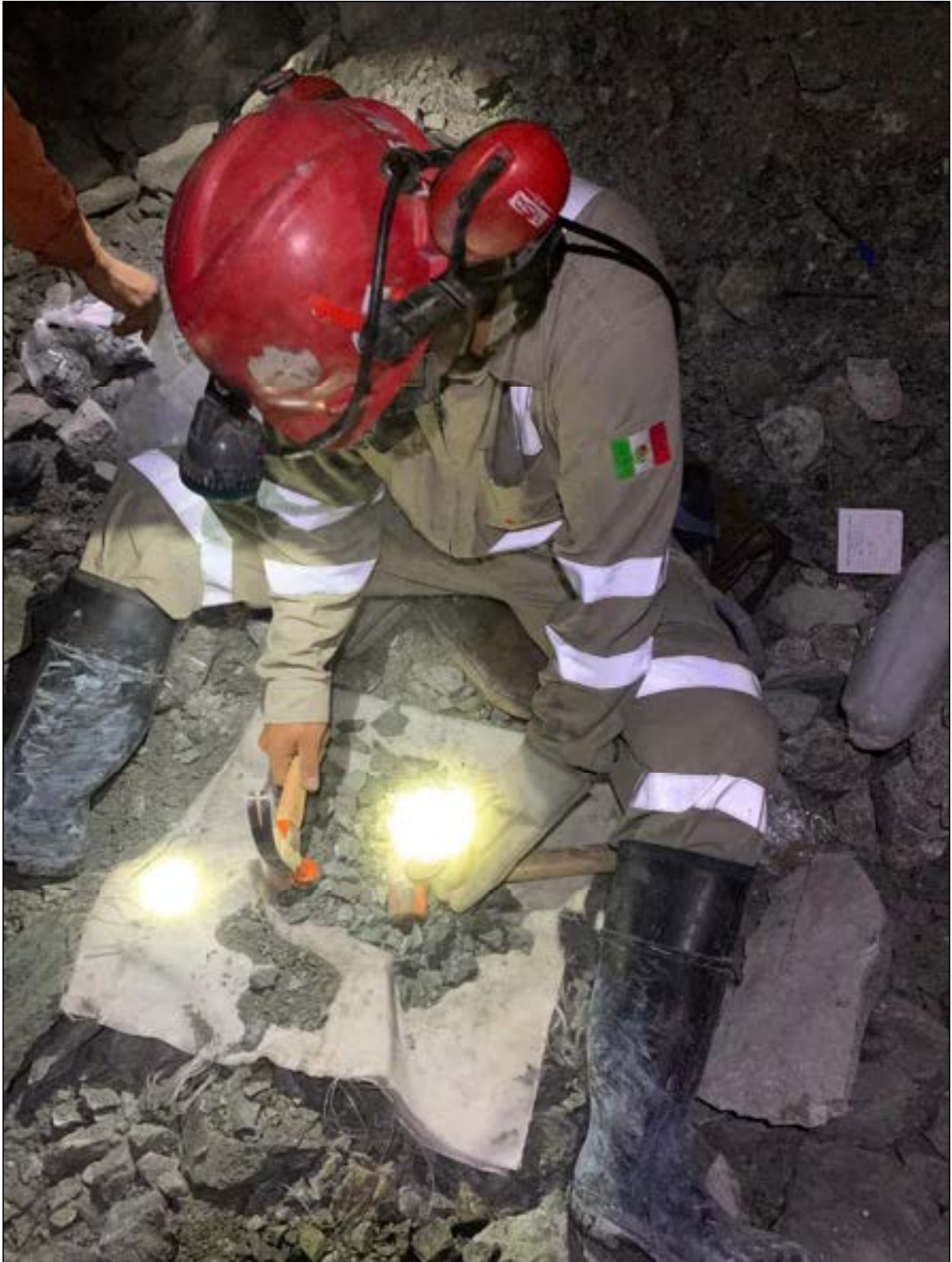
Figure 7-5: Homogenization Process of Sample Particle Size
