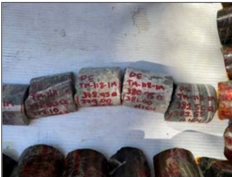
Figure 8.2: Core Samples Selected for Specific Gravity Testing
