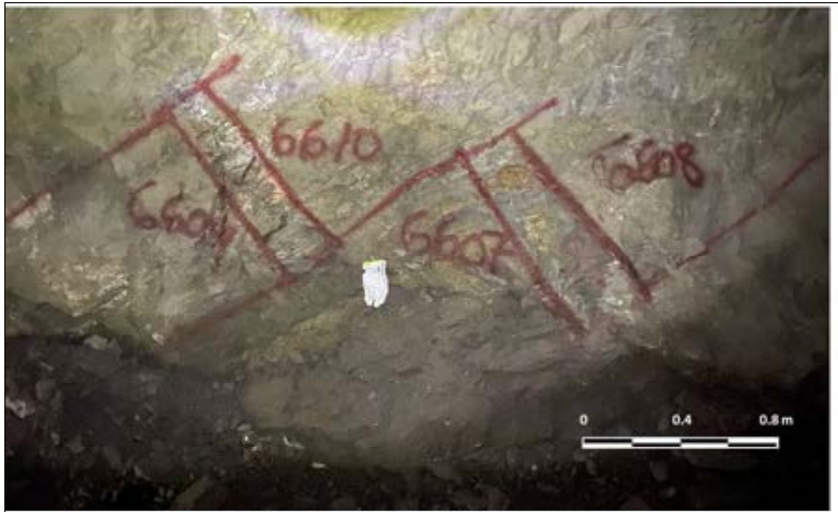
Figure 7-4: Marks Indicating Limits and Width of Samples
