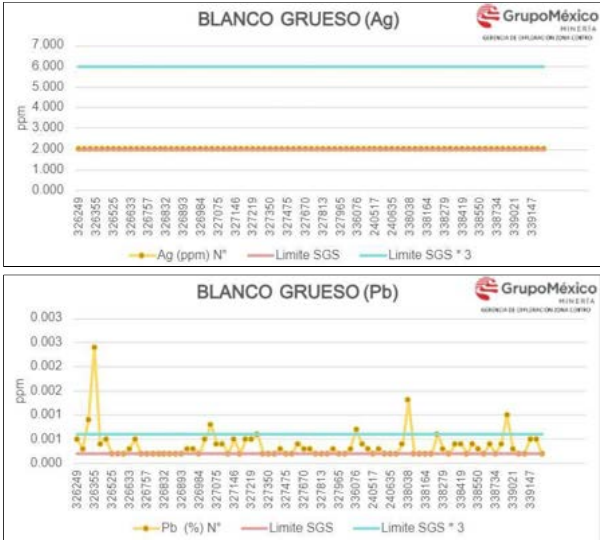
Figure 8-8: Graphs showing the Results of the Coarse Blank Controls (Ag and Pb)
