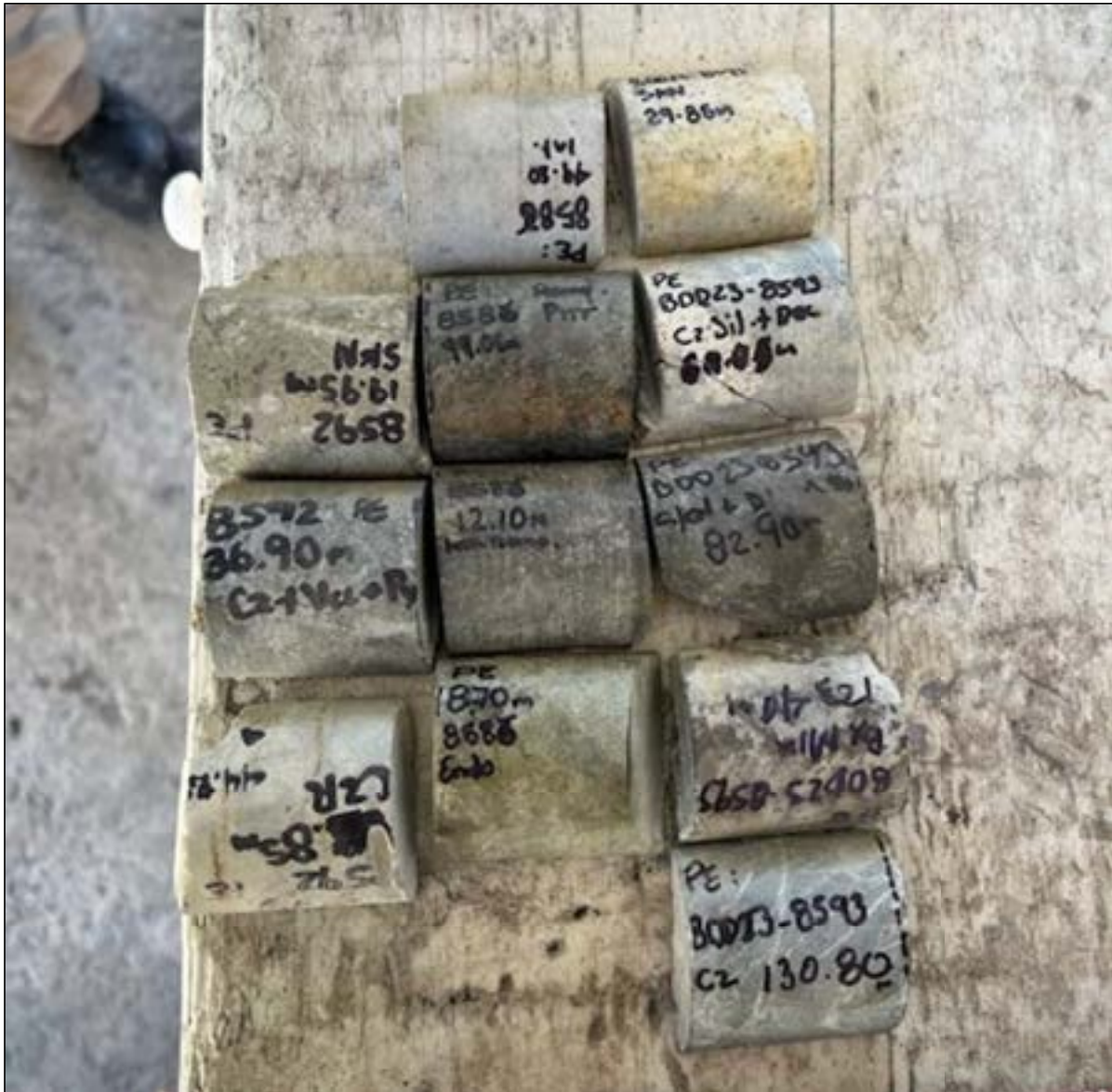
Figure 8-2: Core Samples for Density Testing
