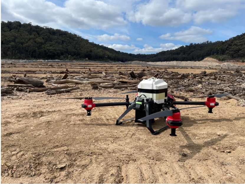
Photo 3 XAG P30 Drone Seeding Trial
