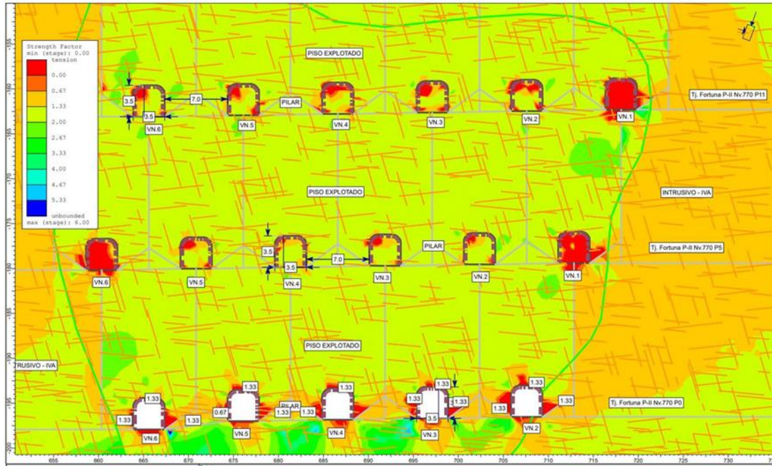
Figure 16-19: RS2 Numerical Model Analysis of Fortuna P-II
