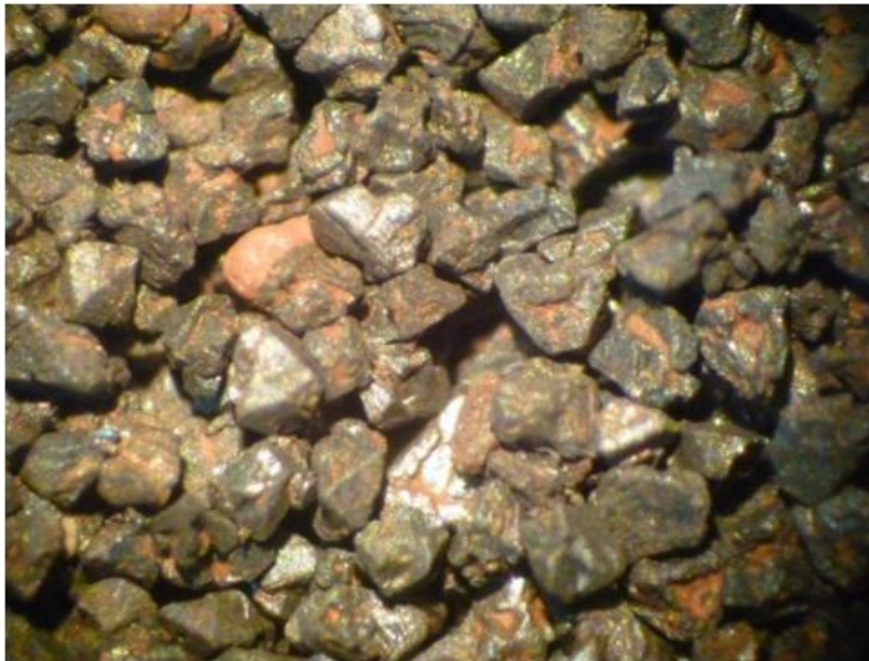
Figure 6-16: Titanomagnetite concentrate with frequent euhedral crystal forms
