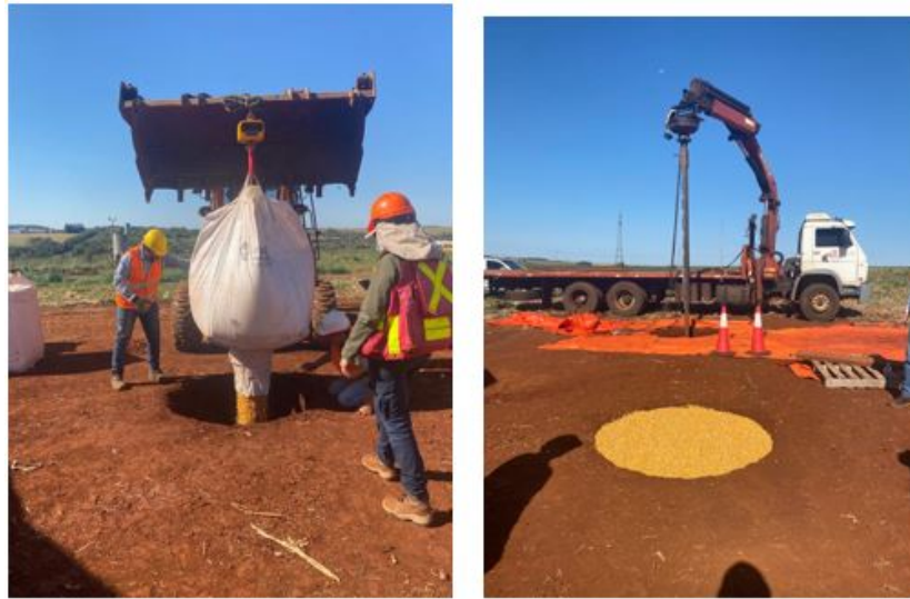
Figure 11-5: Corn grain being poured into one auger hole to measure volume. The lifting scale used to measure the weight of extracted material and replacement corn is visible on the loader
