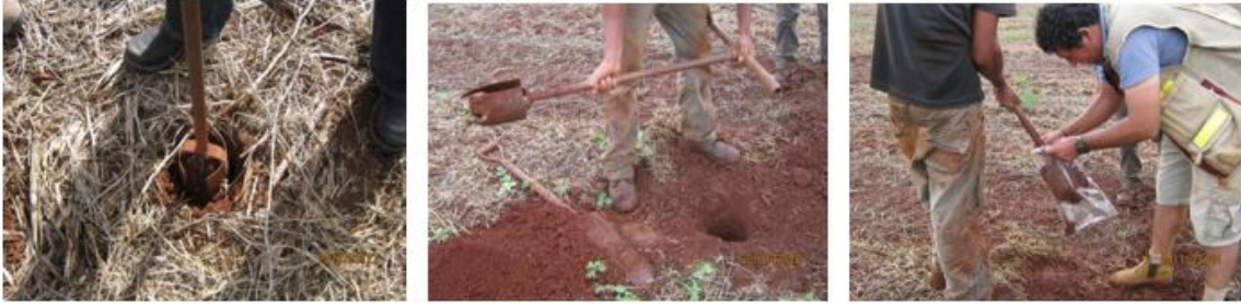
Figure 7-2: Auger sampling at one meter
