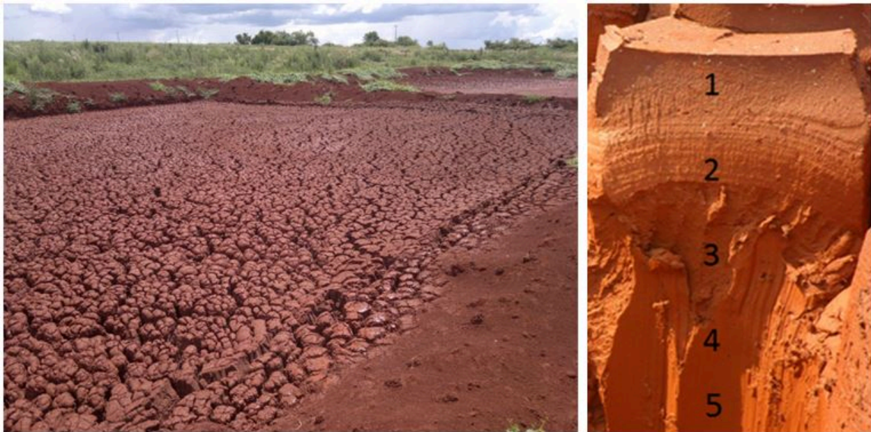
Figure 13-8: 2012 silt/clay tailings drying cell and detail of a clay 'pillar' indicating sample location
