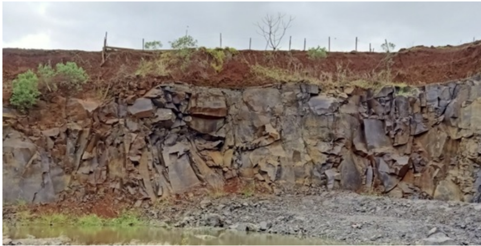
Figure 6-9: Alto Paraná basalt quarry showing overlying laterite
