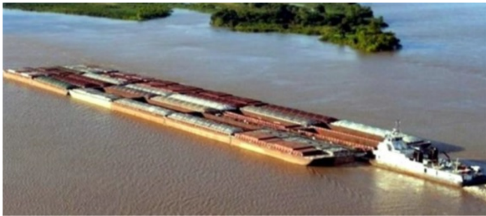
Figure 18-2: Barge transport of loose bulk materials
