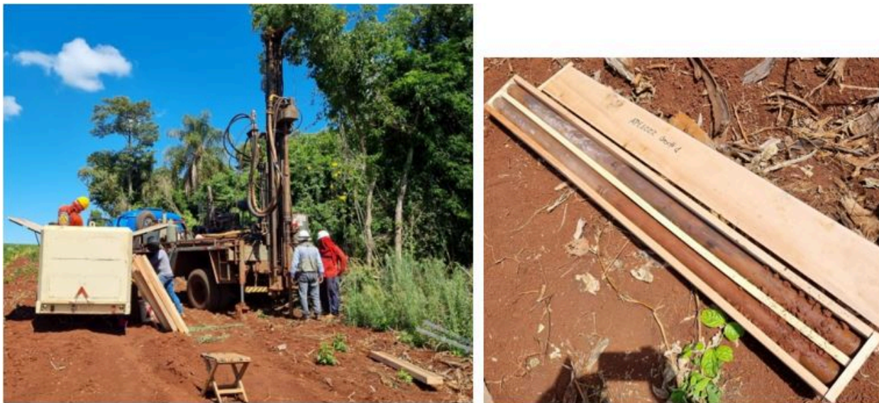
Figure 7-8: 2022 drilling: Geoprobe sampling tool being pushed down with an air-hammer (left) and the recovered sample tubes containing core (right)
