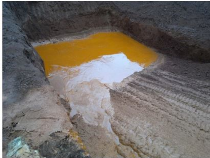
Figure 13-6: Consolidating tailings showing bleed water
