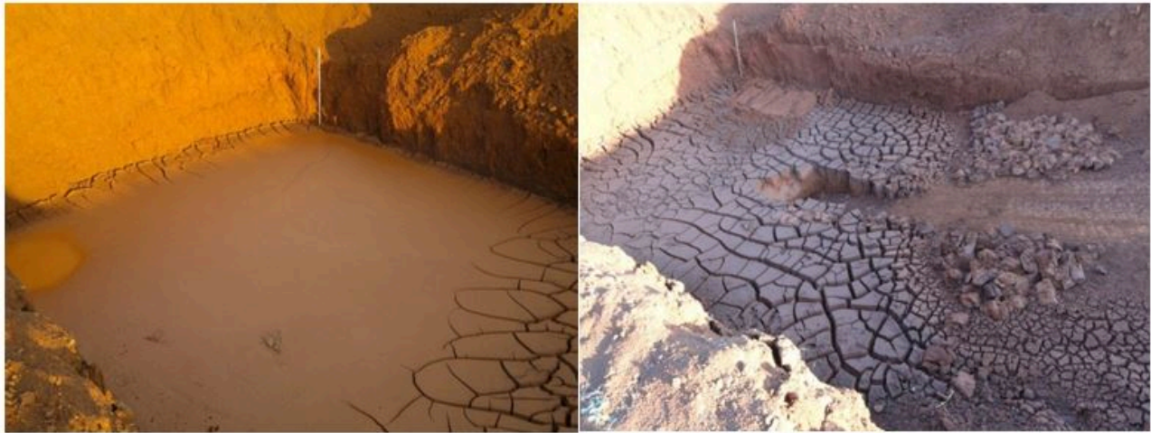
Figure 13-7: Solar drying/shrinkage testing on site showing three months of drying
