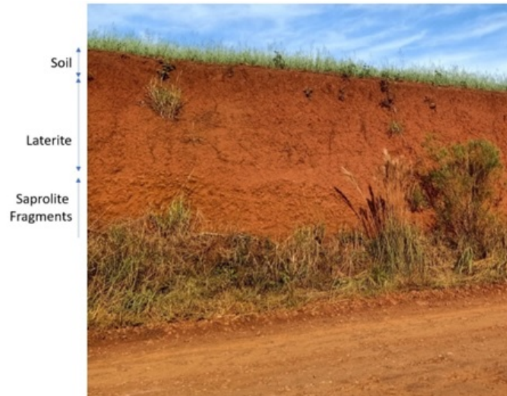
Figure 6-8: Top portion of the laterite profile exposed in a road cutting, Block A Alto Paraná
