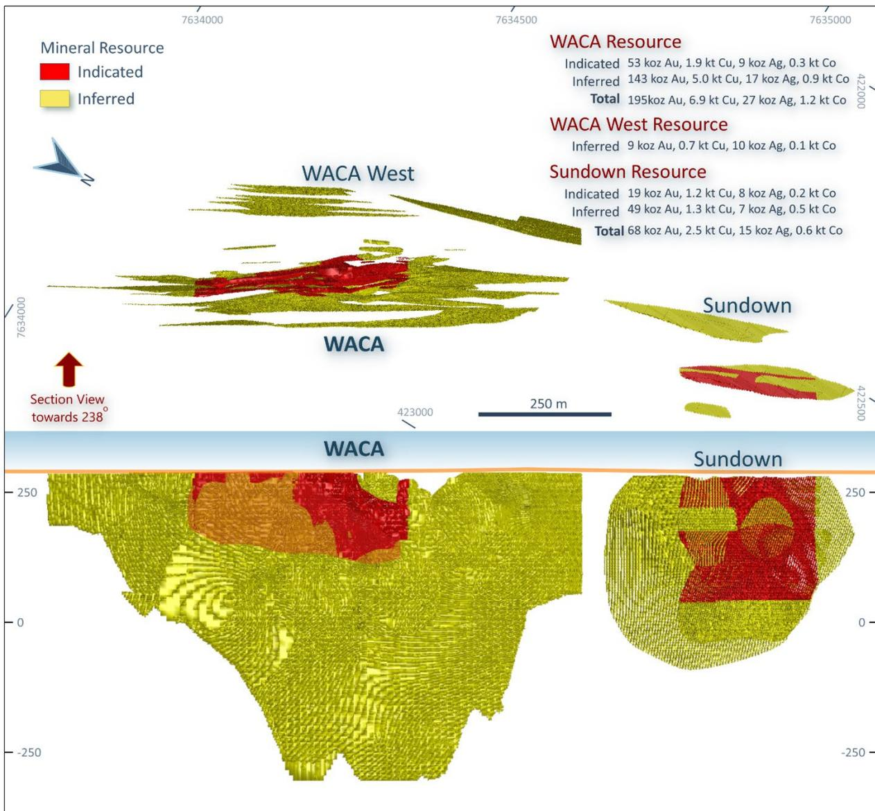
**Figure 7: WACA, WACA West and Sundown deposits Plan and Long Projection views showing distribution of gold-copper-silver-cobalt Indicated and Inferred Mineral Resource.** NB: Regional GDA2020 / MGA Zone 51 co-ordinates, with 500m plan grid and 250m vertical grid, main Long Projection looking horizontally toward Local Grid bearing 270° (or 238° MGA Zone 51).
