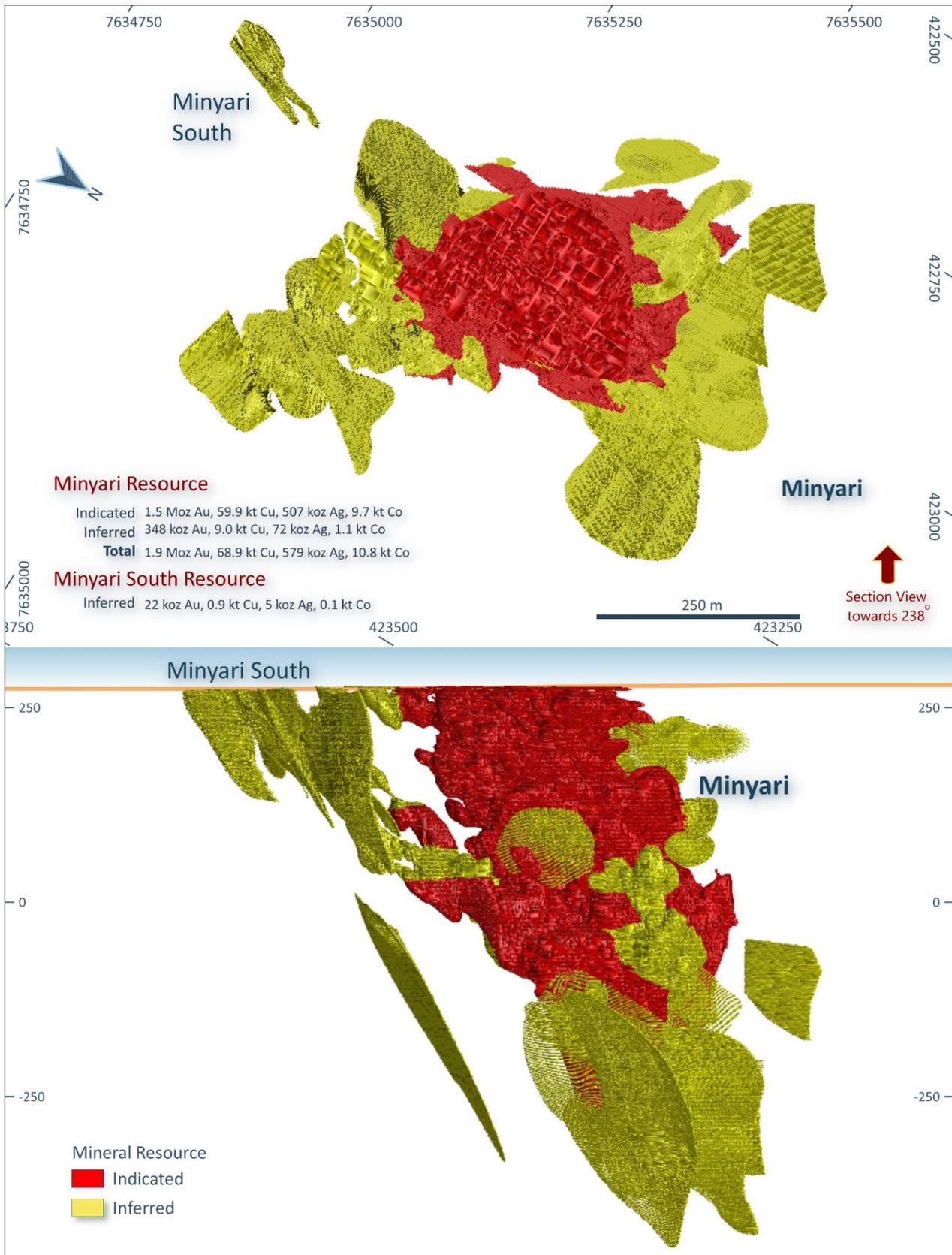
**Figure 5: Minyari and Minyari South deposits Plan and Long Projection views showing distribution of gold-copper-silver-cobalt Indicated and Inferred Mineral Resource.** NB: Regional GDA2020 / MGA Zone 51 co-ordinates, with 250m plan grid and 250m vertical grid, main Long Projection looking horizontally toward Local Grid bearing 270° (or 238° MGA Zone 51).
