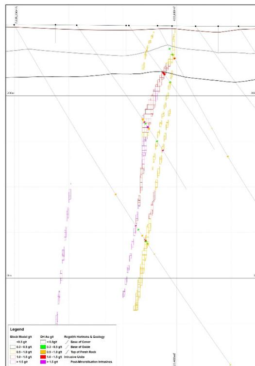
**Figure 13: Sundown deposit cross-section Local Grid 100,800mN, looking Local Grid north (MGA Zone 51 Bearing 328°), showing estimated gold grades in Mineral Resource block model and drill holes showing gold grades. The grid squares represent 200m.**
