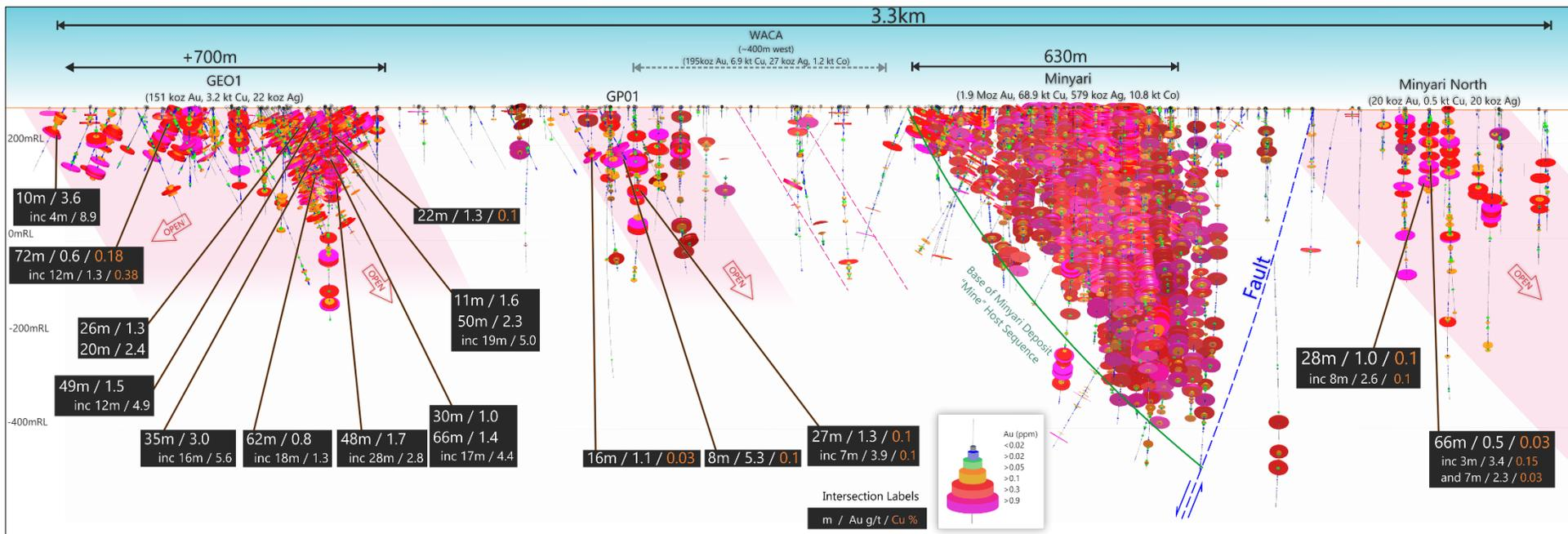
**Figure 9: Long Section from GEO-01 to Minyari North including Minyari and GP01 showing gold drill intercepts and interpreted key features including multiple zones of plunging gold-copper mineralisation. Note the highly prospective 3.3km trend which extends to 4.6km including the Judes copper-silver-gold deposit. NB: 200m elevation (RL), looking toward Local Grid 270° (or 238° MGA Zone 51 Grid).**
