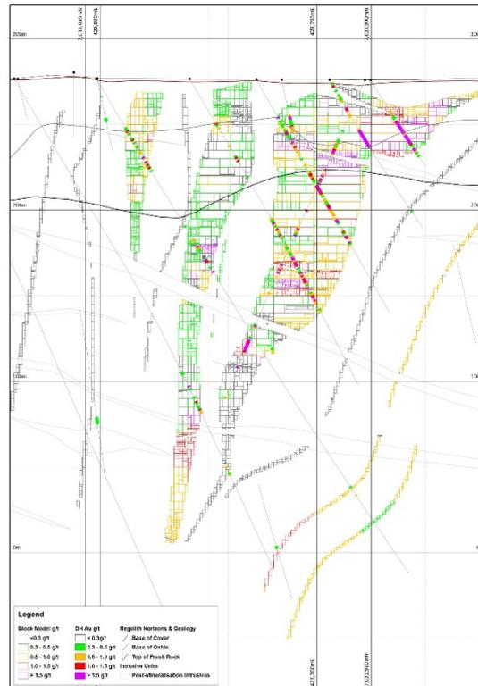
**Figure 12: GEO-01 deposit cross-section looking MGA Zone 51 Bearing 210°, showing estimated gold grades in Mineral Resource block model and drill holes showing gold grades. The grid squares represent 100m.**
