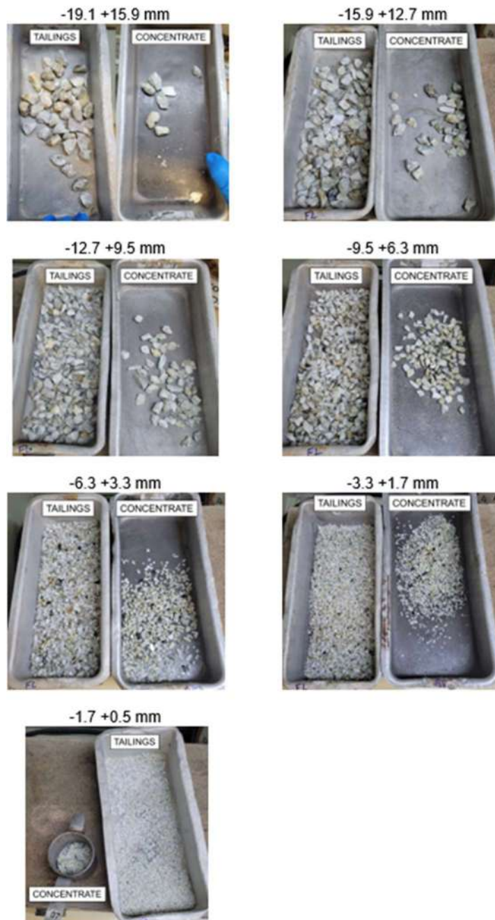
Figure 13-24 – HLS Separation for Rougher Stage
