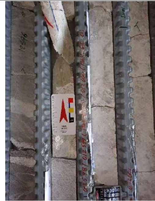
Core boxes of the modelled mineralized spodumene zone – ITDD-23-210 – 220m depth, detail of the Spodumene crystal
