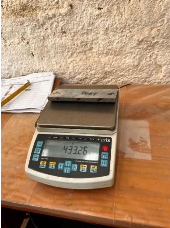
Density measurement – dry core weight
