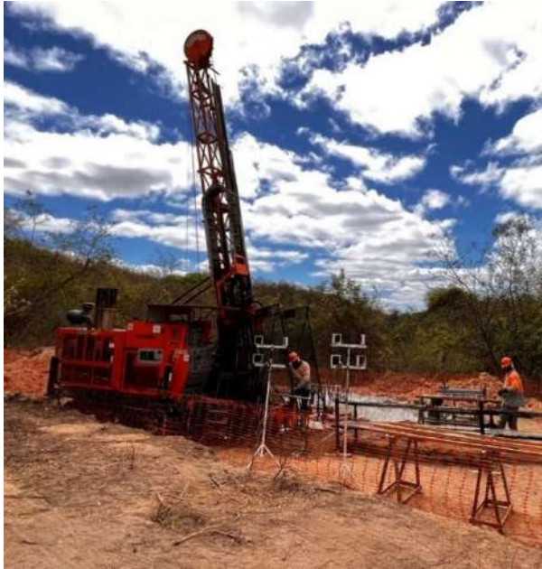
Drill Rig on site of the Bandeira, drilling in 13/09/2023 the DDH ITDD-23-192 - azimuth 140 – dip ~70
