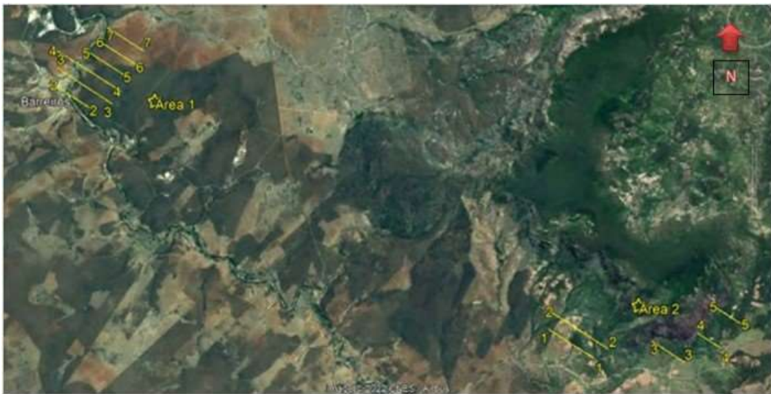
Figure 9-7 – Location of the Lines and Measuring Stations of the Chargeability and Resistivity Data of Area 1 and Area 2 of the Lithium Project
