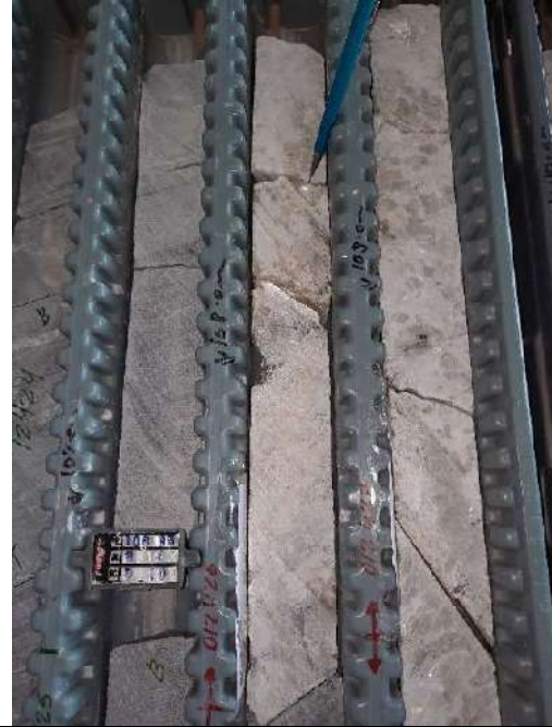
Core boxes of the modelled mineralized spodumene zone – ITDD-23-235 – 108m depth, detail of the Spodumene crystal
