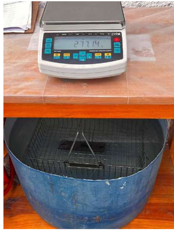
Density measurement – core weight underwater
