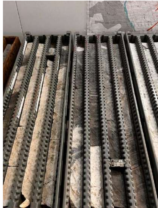
Core boxes of the modelled mineralized spodumene zone – ITDD-23-091 – 479m to 489m
