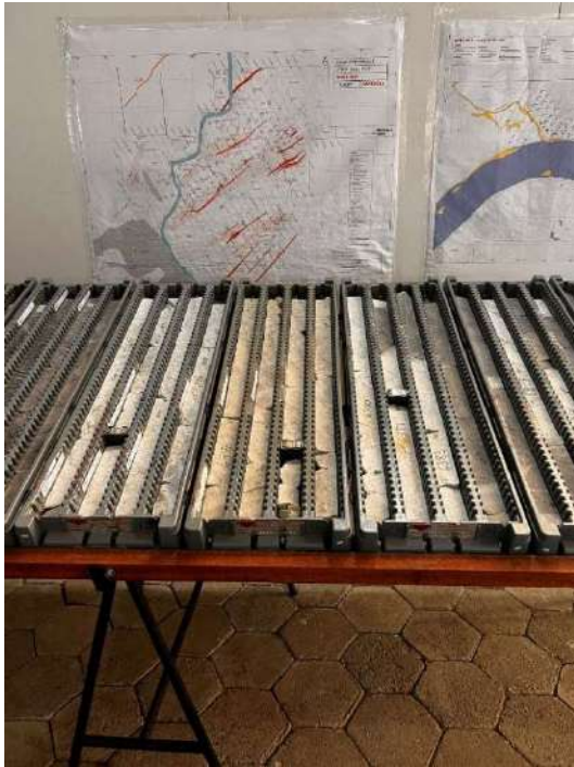
Core boxes of the modelled mineralized spodumene zone – ITDD-23-120 – 109m to 115m
