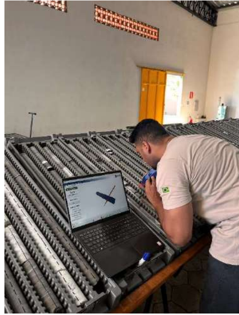
Geologists are doing the structural and geological logs.
