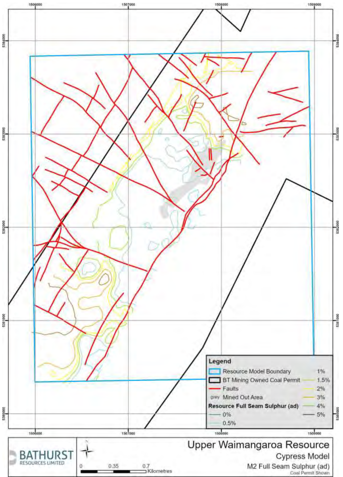
Figure 12: Plan showing full M2 seam sulphur on an air dried basis across the Cypress resource
