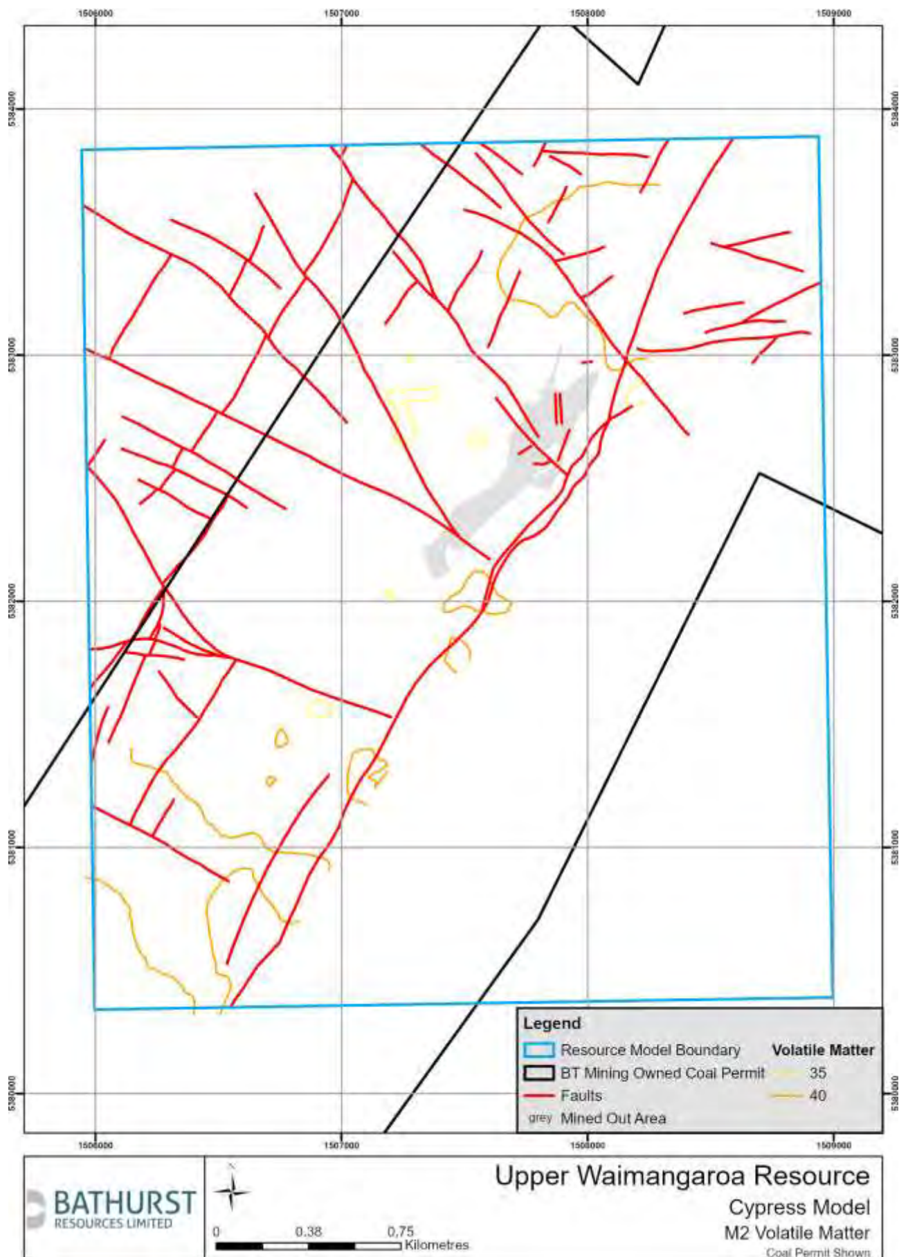
Figure 13: Plan showing full M2 seam Volatile Matter on an air dried basis across the Cypress resource
