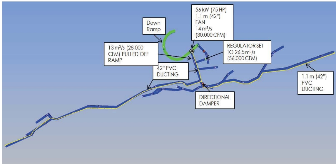
Figure 16.9: Typical Level Ventilation Circuit
