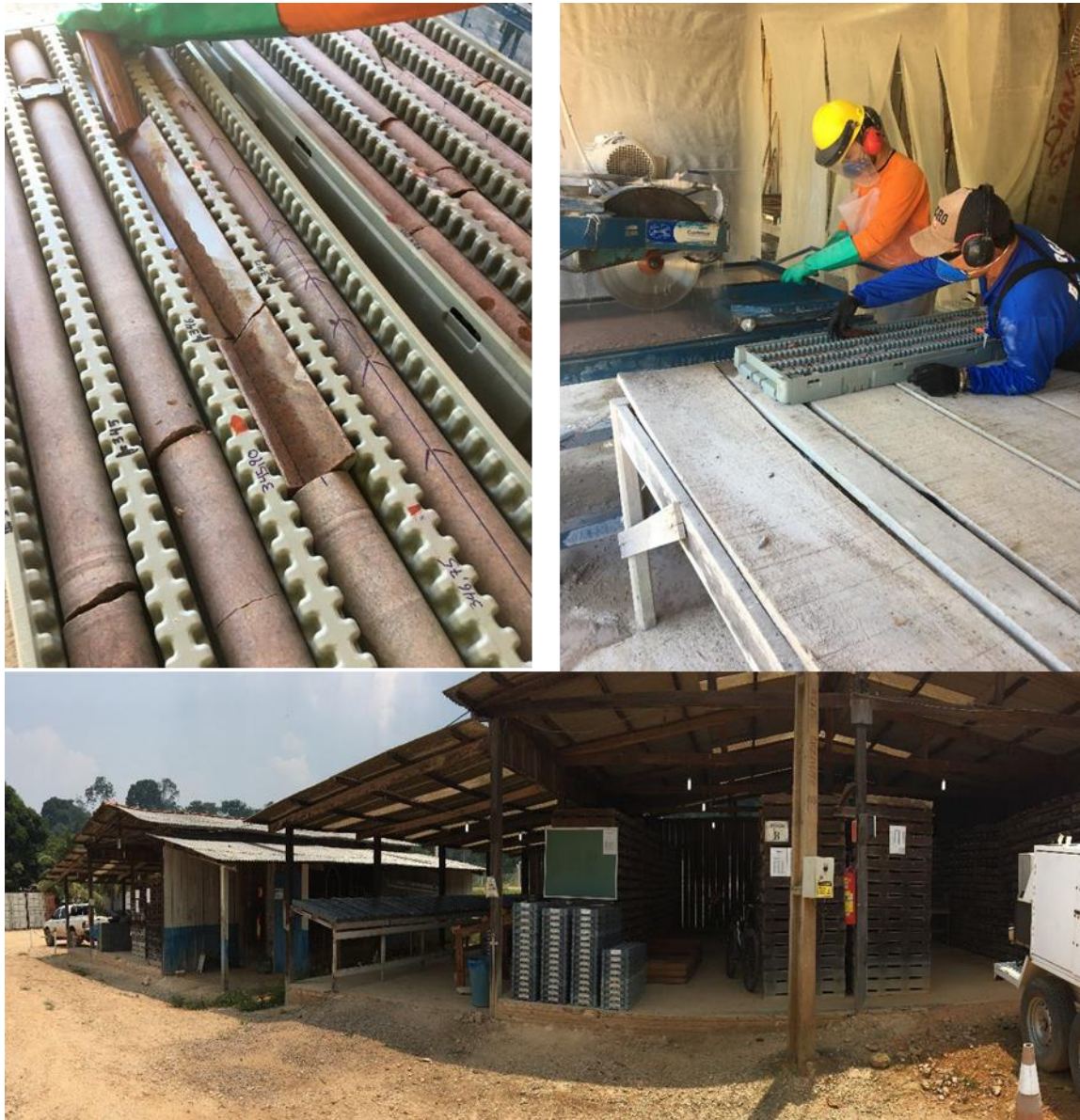
Figure 11-2: Marking Core, Cutting Core, and the Core Storage Facility
