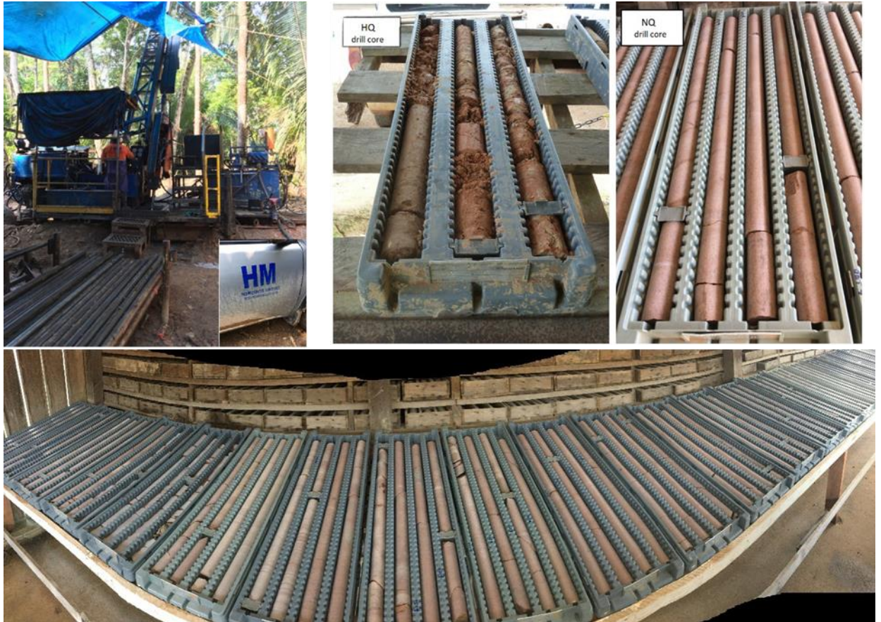
Figure 11-1: Drill Rig, HQ, NQ Drill Cores and a Series of Consecutive Core Boxes
