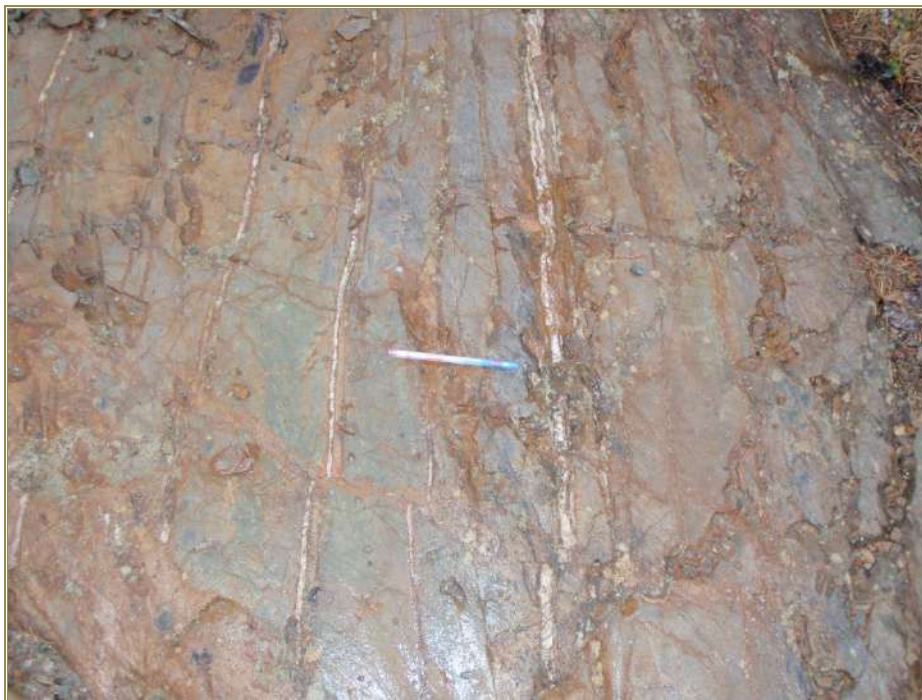
Figure 8-3: Exposure of the Brookbank Deposit Quartz-Carbonate Veining and Fractures
