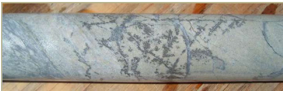
Figure 7-20: Example of Fracture-Controlled Pyrite Mineralization in Sericite-Silica Arkosic Wacke, 0.54 ppm Au
