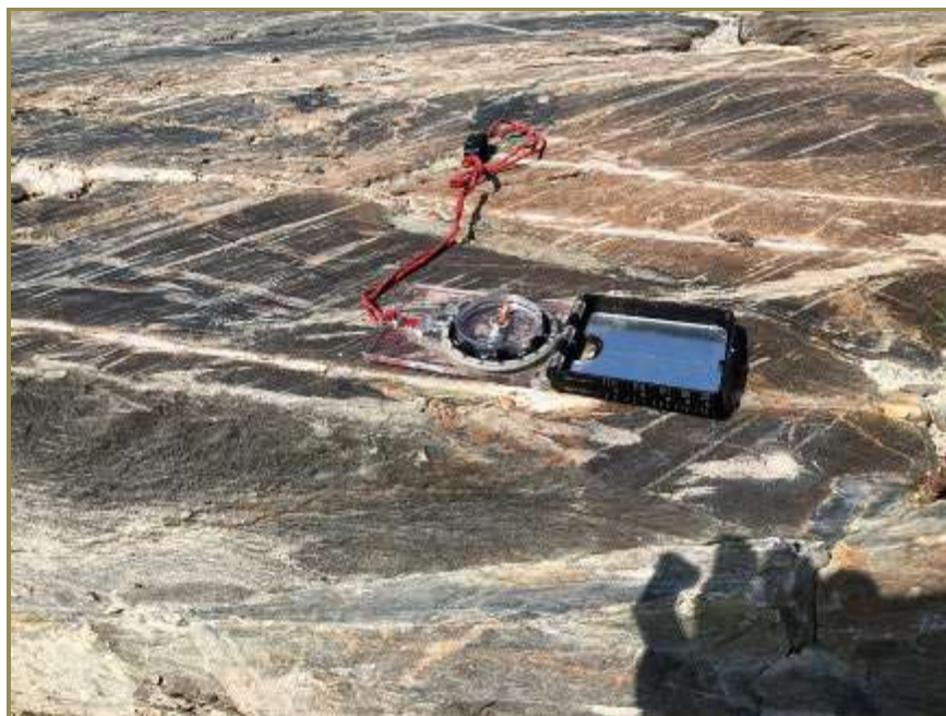
Figure 7-7: Quartz Carbonate Veins and Sericite Carbonate Alteration at the F Zone
