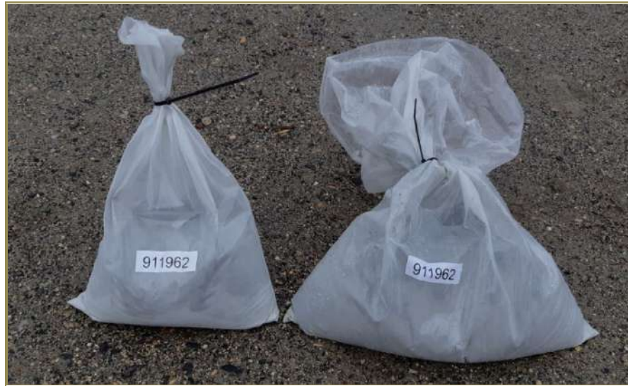
Figure 11-1: Principal Sample (Small) and Metallurgical Sample (Large) from a 2 m Interval—RCGC Sample
