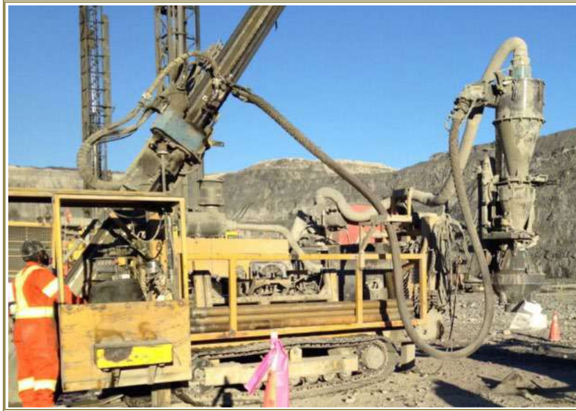
Figure 10-5: Hardab 7000 Maxidrill RC Drill Rig
