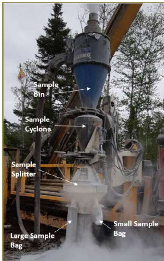
Figure 11-2: Hardab 7000 Maxidrill RC Drill Rig and Splitter in Operation
