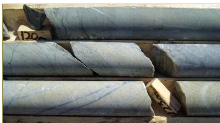
Figure 7-21: Example of Sericite-Altered Quartz-Feldspar Porphyry, 7.75 ppm Au
