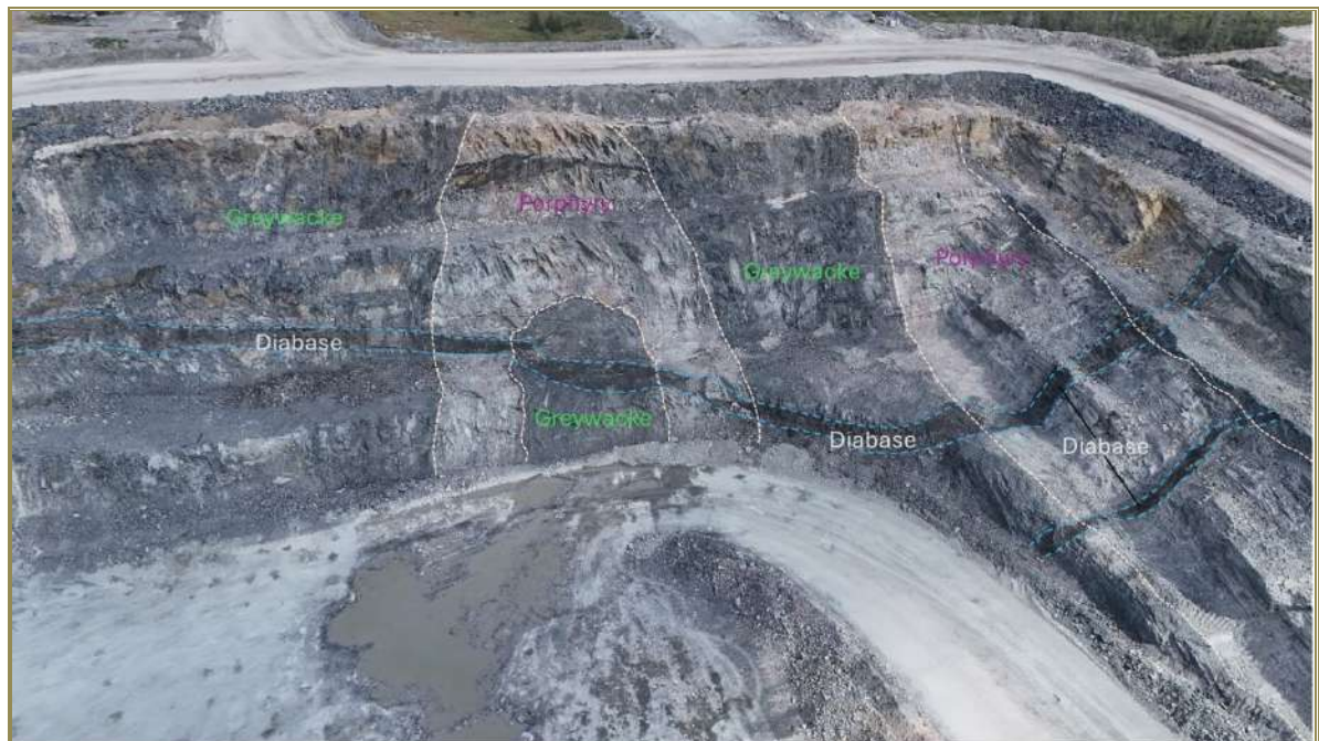
Figure 7-13: Greenstone Mine, East Pit at Southeast Corner—Folded Porphyry and Greywacke Units Crosscut by Younger Diabase Dikes
