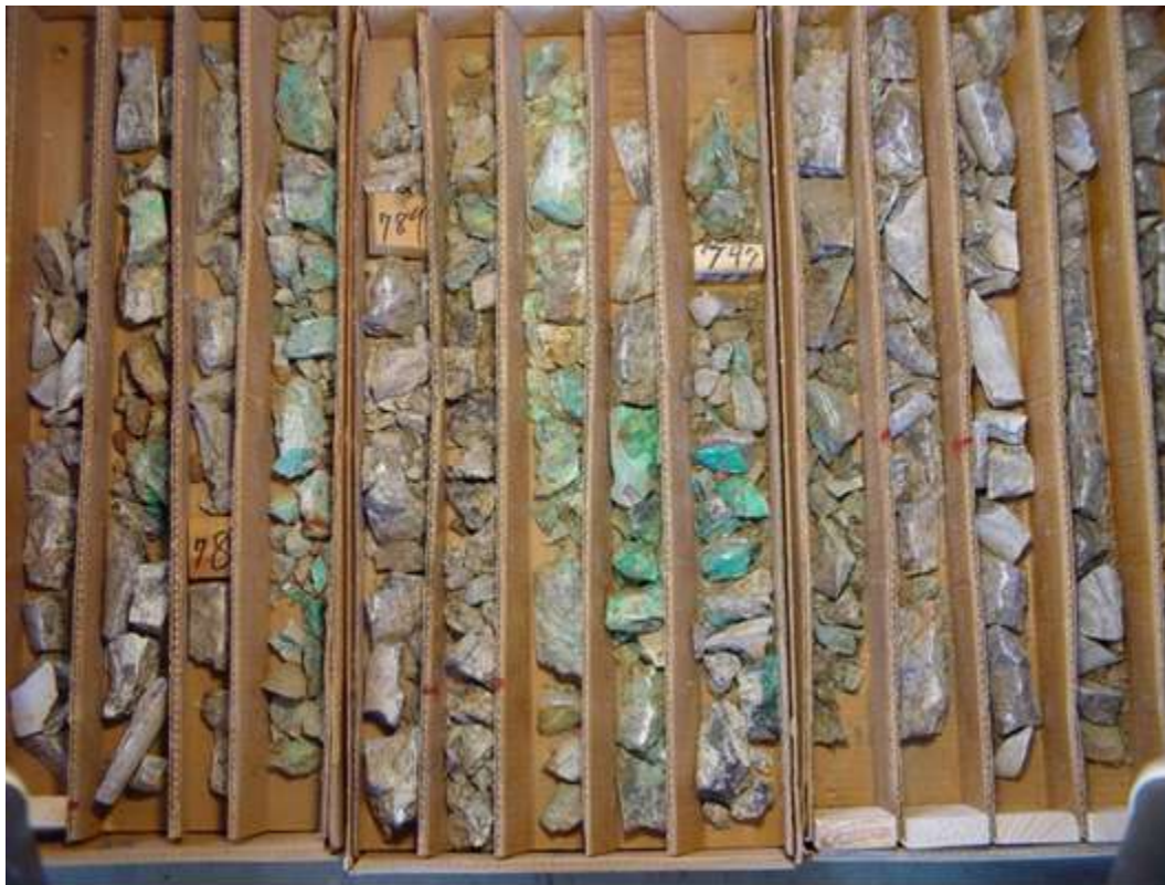
Figure 7-8: Photograph of Typical Oxide Mineralization for the Gunnison Deposit Hole J-9: 780 to 806 feet
