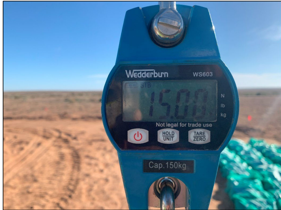
Figure 8: Wedderburn WS603 scale being calibrated to 10kg & 5kg standard weights.
