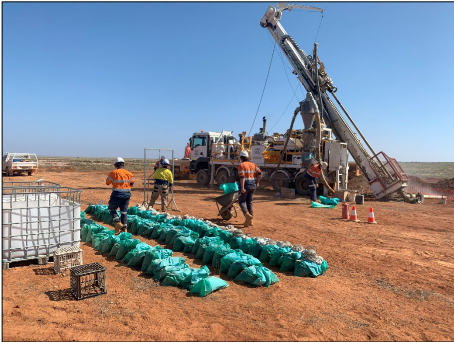
Figure 7: Rig and sampling setup at Drillhole RCFO24011. - Samples are transported from the Metzke cone splitter to the weigh station via wheelbarrow. - Samples laid out in 30m rows ready for hand-held magsus readings. - IBCs at hand for dispatch of primary samples and storage of secondary samples.
