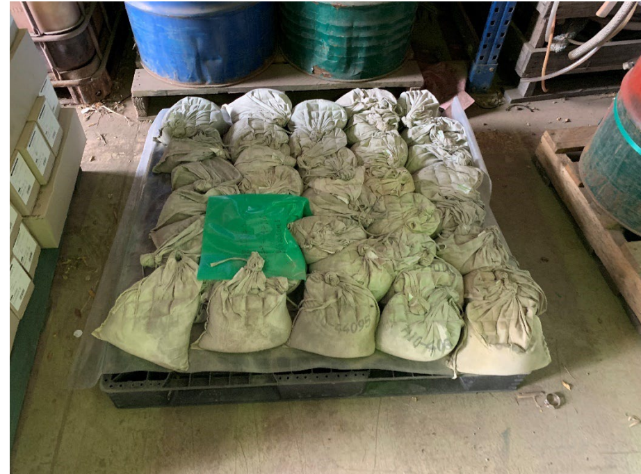
Figure 16: Hawsons 1m RC chip samples awaiting Rotary Sample Division and compositing at BV.
