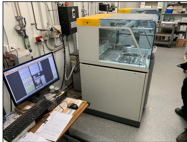
Figure 18: BV's AXIOS 2 DY602 automated XRF assay analyser with borate fusion discs in process.
