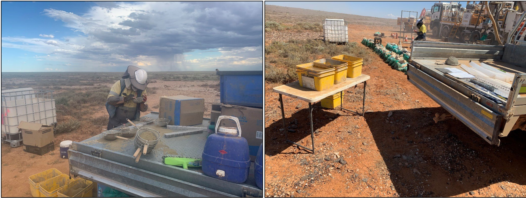
Figure 10: Geologist logging & sampling RC chips into trays on the back of the utility vehicle. Square, yellow pails are filled with water for washing samples.
