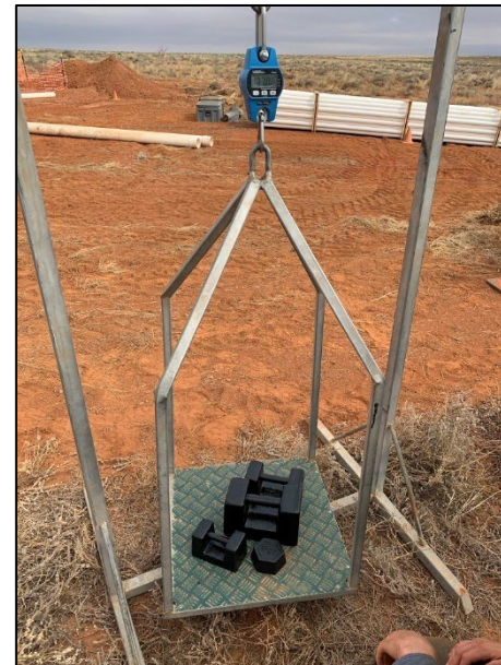
Figure 8: Wedderburn WS603 scale being calibrated to 10kg & 5kg standard weights.
