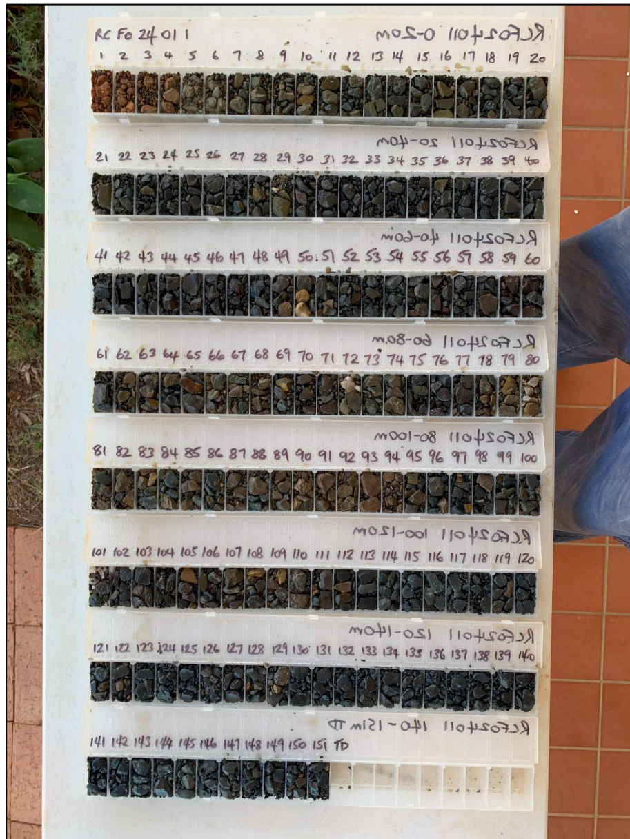
Figure 11: Chips from 0-151m (TD) in drillhole RCFO24011.
