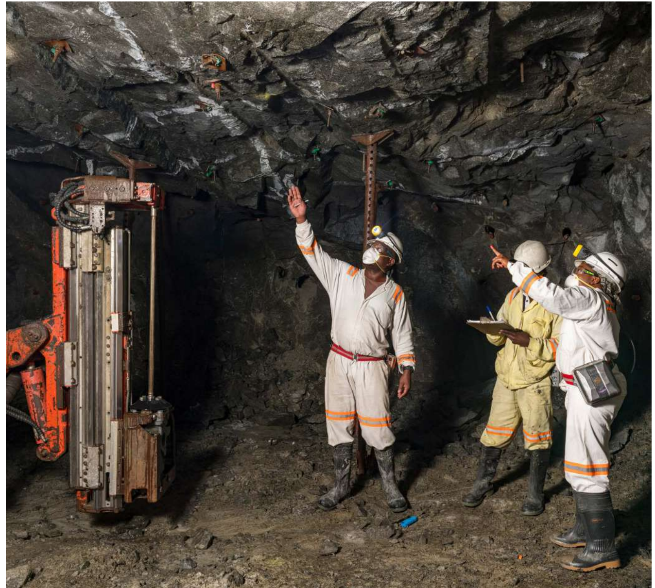
Inspection of the underground hangingwall at Zimplats
