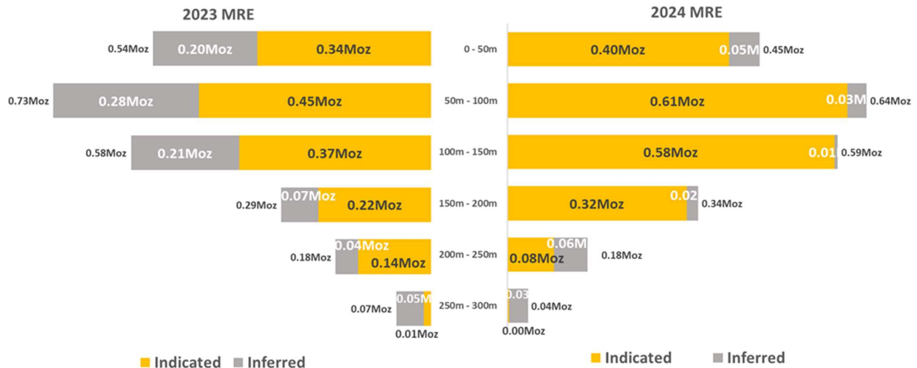
Figure 5: Comparison of Kobada Mineral Resource by level showing Indicated and Inferred Resources
