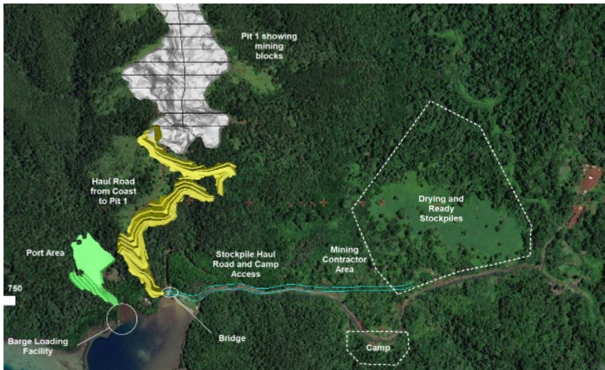
Figure 28 Mine and Operations Site Layout
