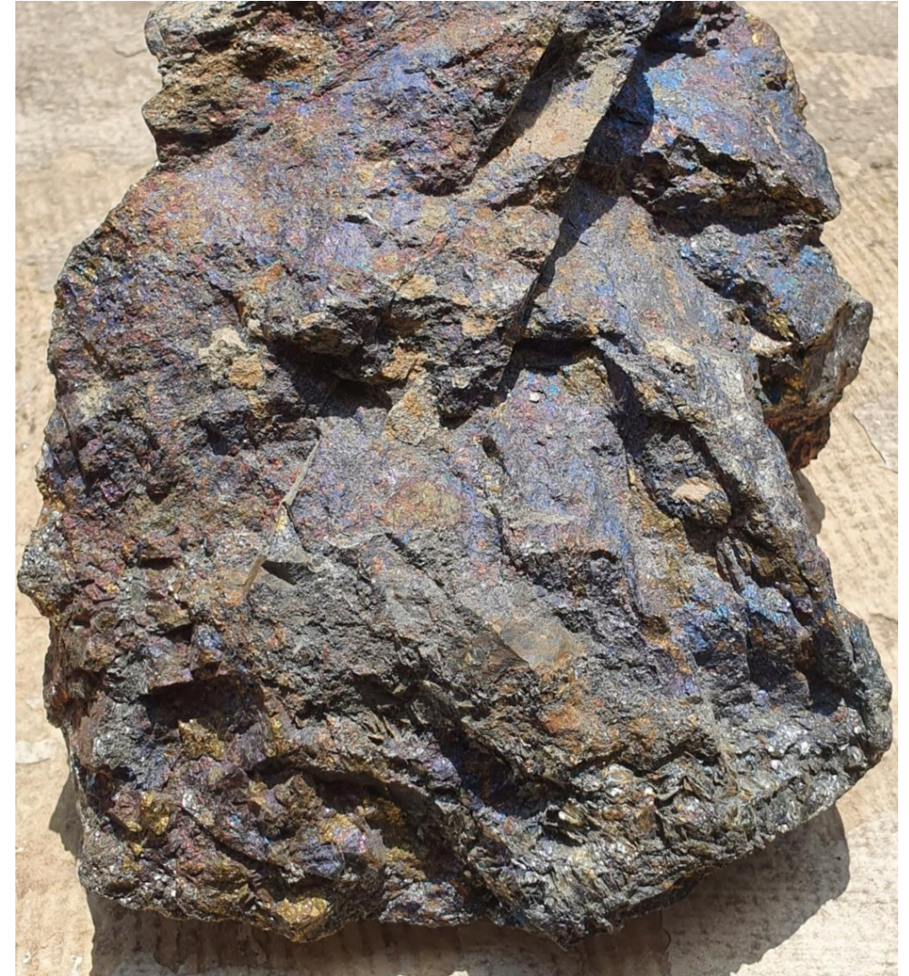
Left: Stringers of silvery-golden Co-Ni mineralization in low grade metamorphic sediments (gray) from the waste dump of G7.
