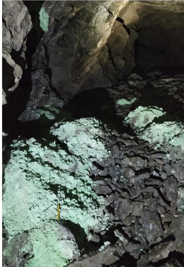
Below: Powdery, greenish nickel oxide minerals on the wall of G7 and rocks on the gallery floor. Yellow magnetic pen for scale.
