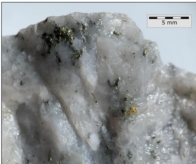
Figure 10-2: Visible Gold Hosted in Quartz Vein from Drill Hole FG20-002C at 47.25 m, the Sample C375828 from 47 – 48 m Returned 14.45 g/t Au.
