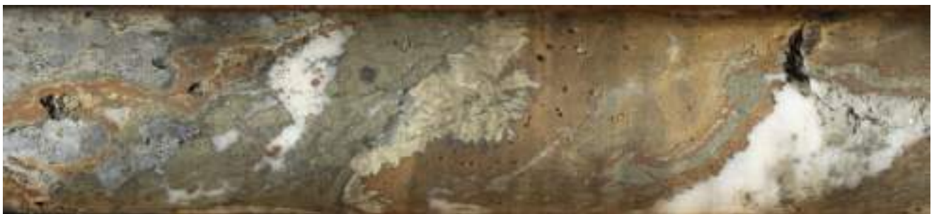
Figure 7-22: Boundary Zone Vein Mineralization NB23-029 Core Photo
