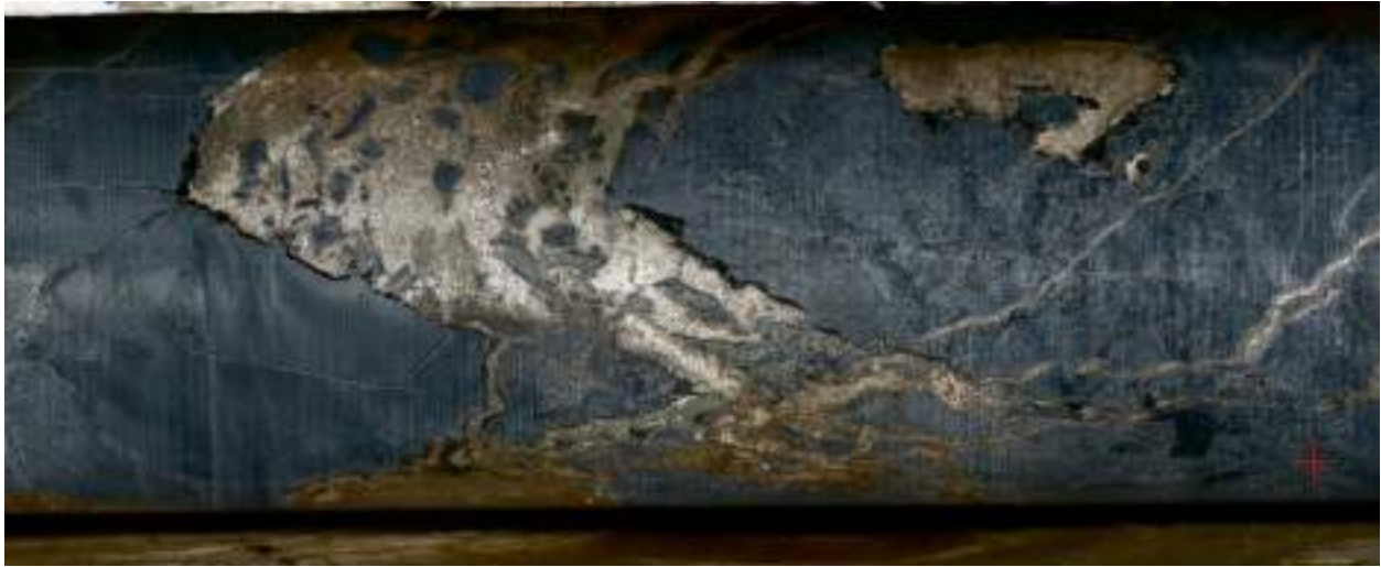
Figure 7-23: Hydrothermal Sphalerite Breccia Developed Along a Stylolite, Boundary Zone
