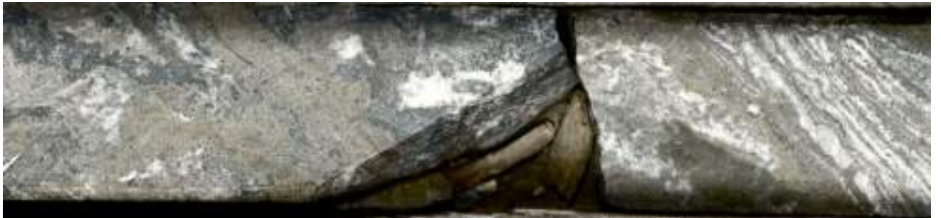
Figure 7-13: Quartz-Sulphide Facies from JS81-068W1
