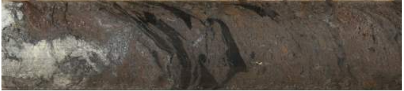
Figure 7-6: Massive Sulphide Feeder Facies from TS23-009
