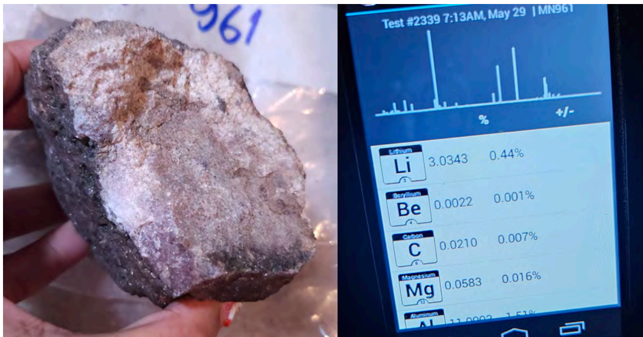
FIGURE 8: SPLA01/2566 – 6.51% Li 2 O with a LIBS reading of 3.03% Li (Test #2339 below), is a new discovery (Pink Panther North) approximately 1.5km to the northwest of Matsa’s Pink Panther prospect.
