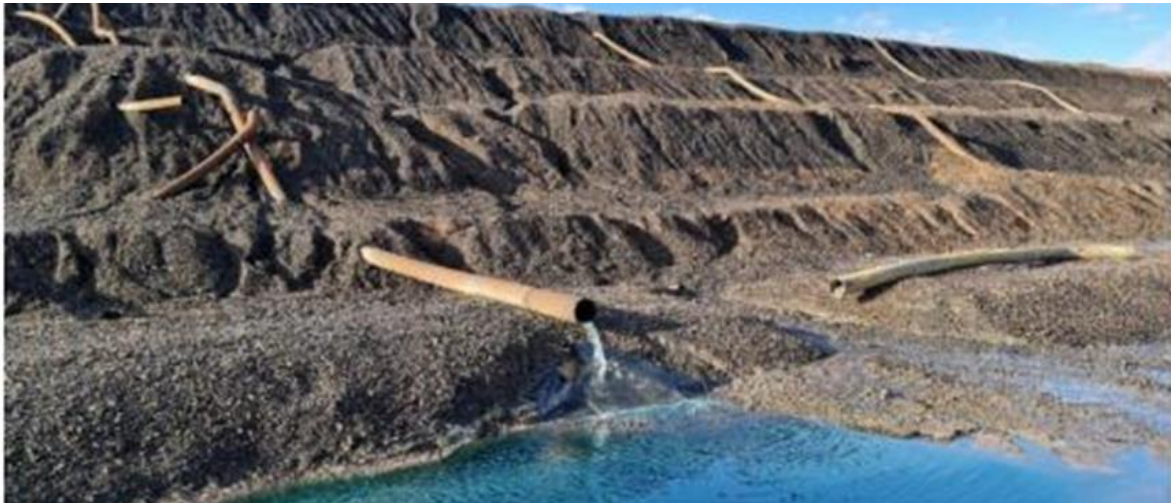
Figure 3 – Copper Solution Flowing out of Existing Heap Leach Pads
