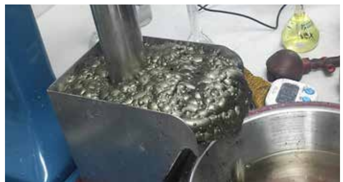
Photo 7: Photograph showing a batch flotation test of the PCZM supergene ore at Maelgwyn.
