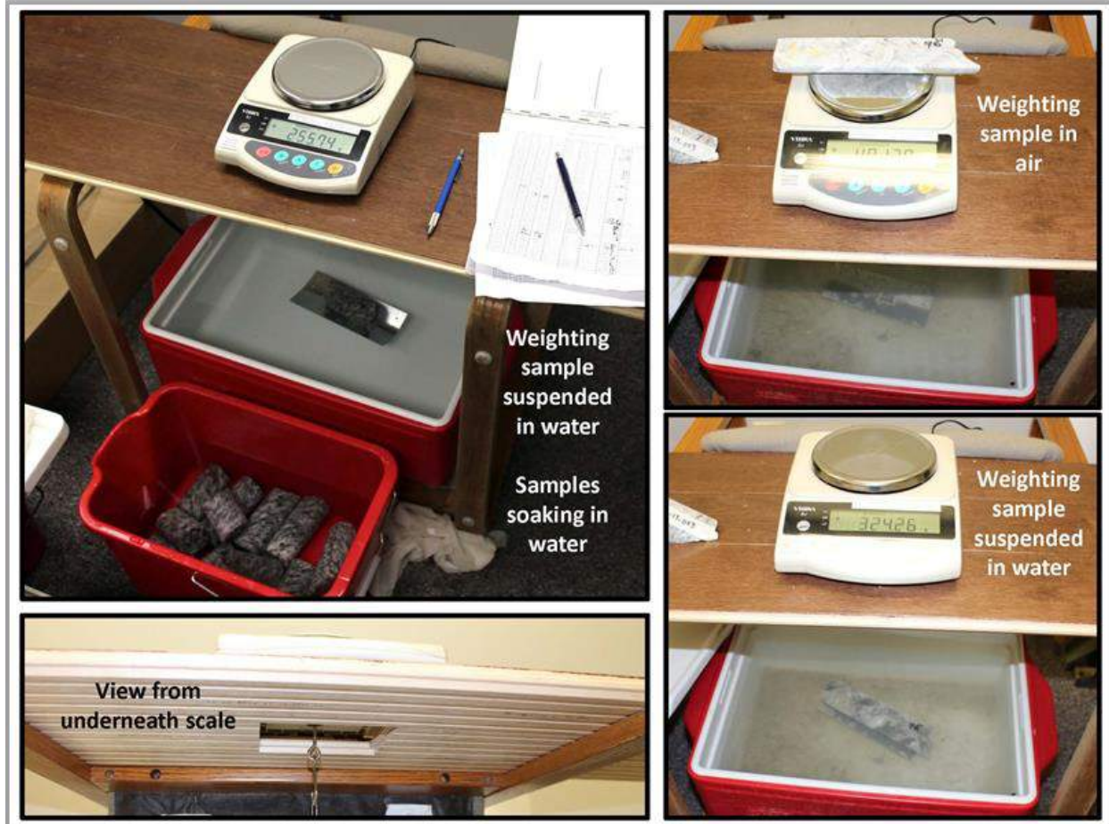
Figure 14-1: Specific Gravity Station
