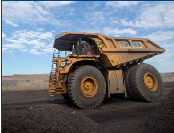
Plate 2 – Trucks Used for Overburden Removal at the Peak Downs Mine
