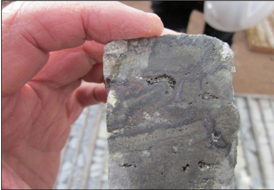
Figure 7.7: Crustiform Texture in HQ Core (~63.5 mm Width) - Pulacayo
