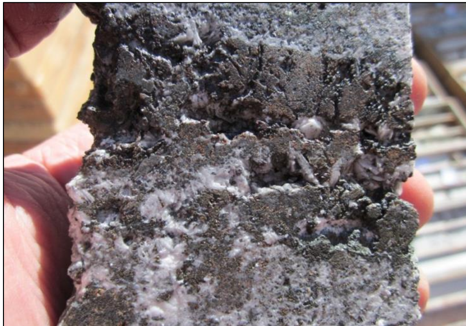
Figure 7.8: Vuggy Quartz and Barite in HQ Core (~63.5 mm width) – Pulacayo
