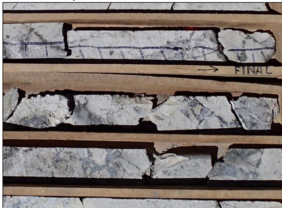
Figure 7.11: Breccia Hosted Style Mineralization – Paca Hole 092 at ~ 47m
