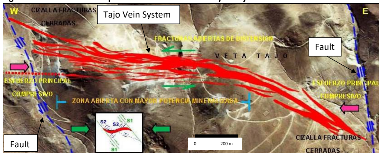
Figure 7.5: Structural Interpretation For TVS at Pulacayo Project
