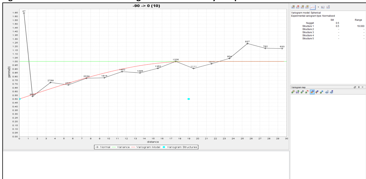
Figure 14.15: Downhole Zinc Variogram for the Pulacayo Deposit
