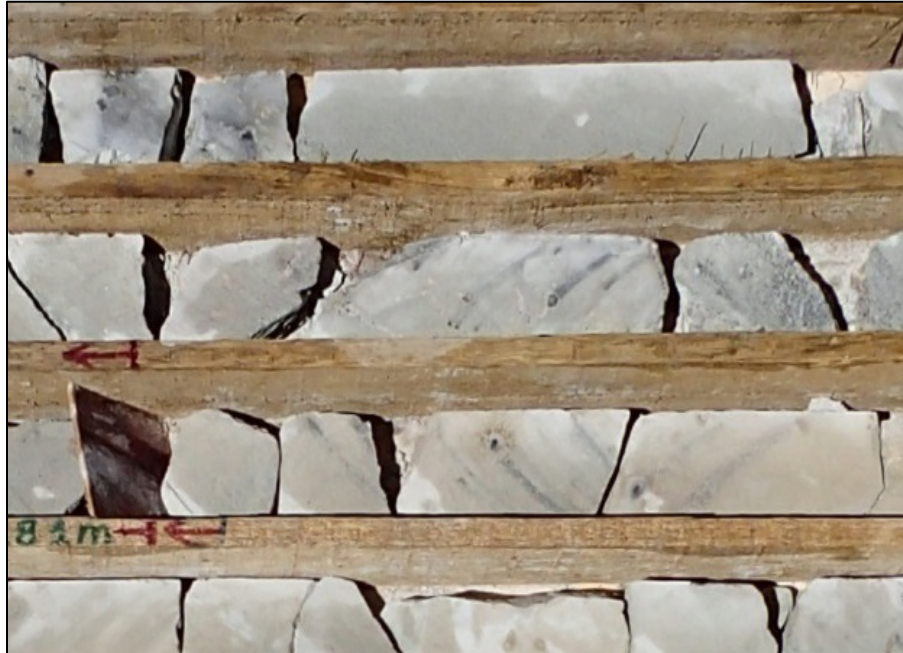
Figure 7.10: Disseminated Mantos Style Mineralization - Paca Hole PND-061 at ~180m
