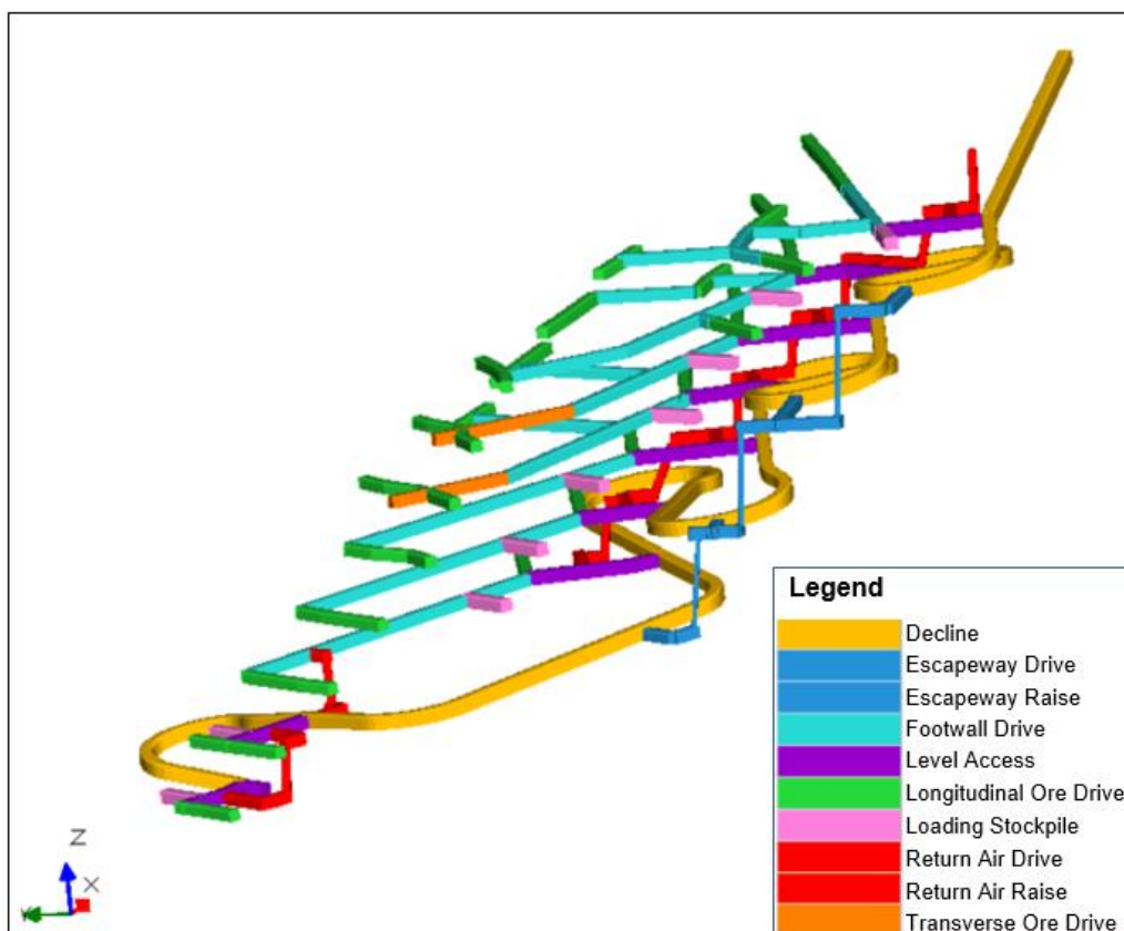
Figure 16-28: Oblique view of Rumajärvi mine development design
