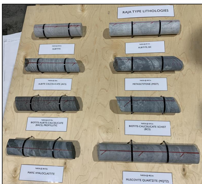
Figure 16-5: Representative core of the main lithology types (Mawson Site)
