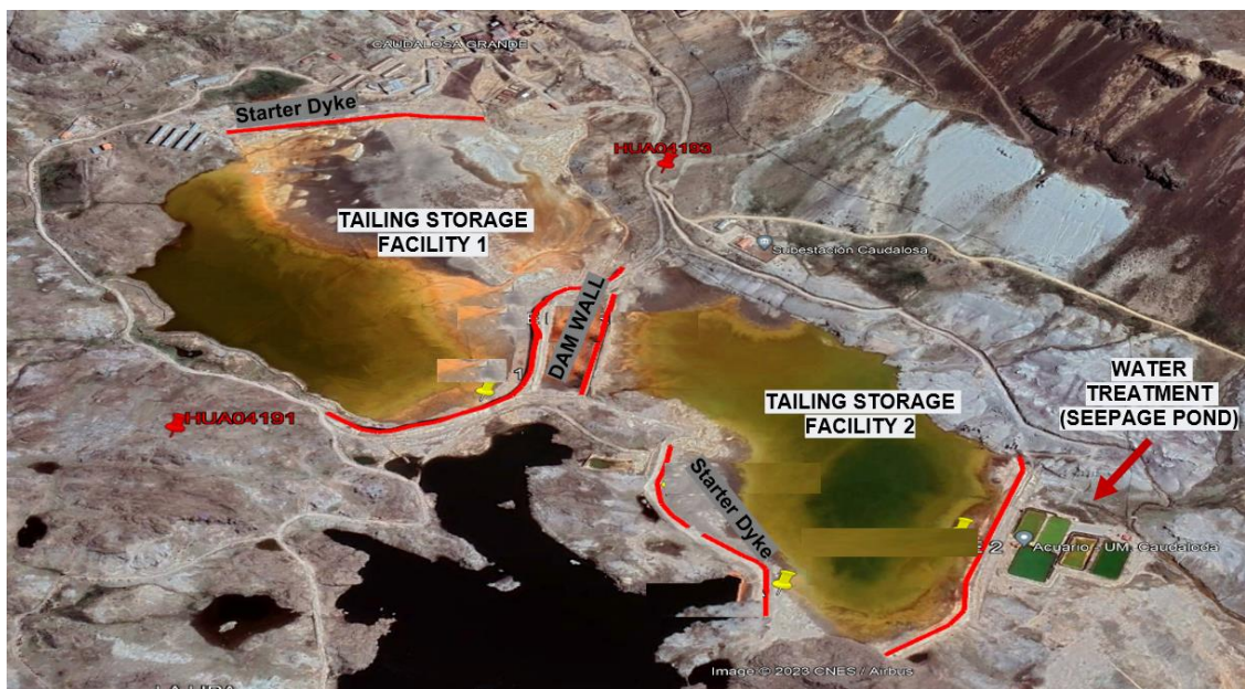
Figure 18.5 Satellite image of components of tailings storage facilities (TSF-1 and TSF-2), Reliquias Mine
