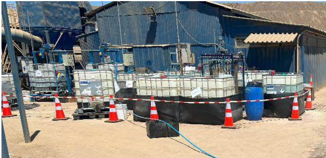
Figure 13-9: Pilot Ion Exchange Circuit at Mantoverde for The Recovery of Synthetic Cobalt Solutions.
