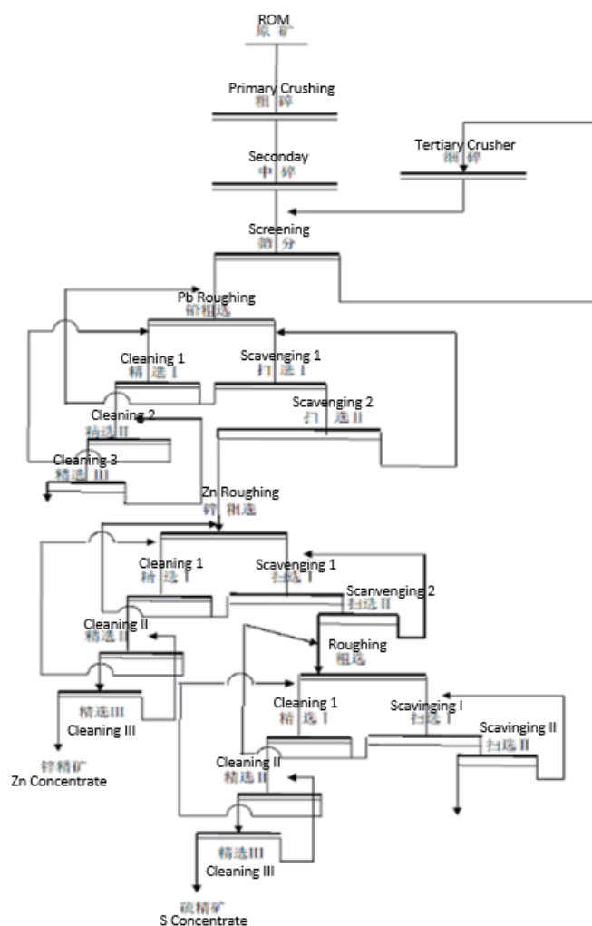
Figure 5-11 2,000 t/d Processing Flowsheet Diagram
