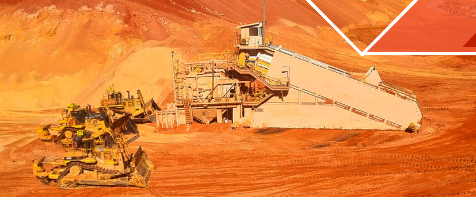
Figure 2 Coburn Project – Dozer Push Mining of Free-flowing Sand
